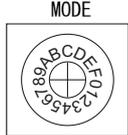
The MODE switch is a rotary switch with positions labeled 0, 1, 2, 3, 4, 5, 6, 7, 8, 9, A, B, C, D, E, F.
