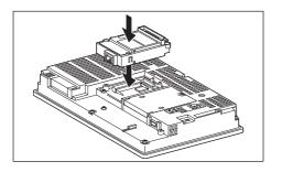
Mount the Ethernet communication unit on the extension unit connector of the GOT.
