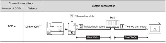
\*1 Connect the GOT to the Ethernet module via a hub.
