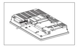
Connect the twisted pair cable to the Ethernet communication unit. OVERVIEW
