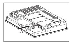
Connect the twisted pair cable to the GOT Ethernet interface.
