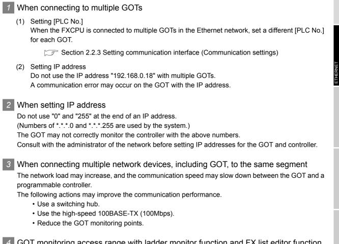
4 GOT monitoring access range with ladder monitor function and FX list editor function The GOT can access only the target CPU with the ladder monitor function and FX list editor function. The GOT cannot monitor the other stations.
