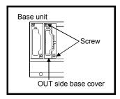
Loosen the screw on the OUT side base cover of base unit.
