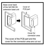
) A9GT-QCNB is installed on the QA1S6□B type base unit Please cover of the substrate part, cover for the connector area, and cut out the detached base cover.
