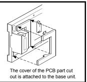
The cover of the substrate part cut out is attached to the base unit again.
