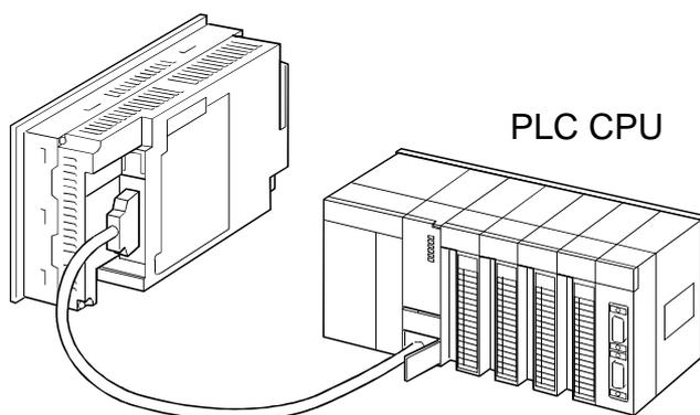
When bus connection communication board is used, it is necessary to set the increased number of stages and the I/O slot number.
