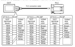
User-made cable is necessary, depending on the PLC. For the detail, refer to GOT2000 Series Connection Manual.
