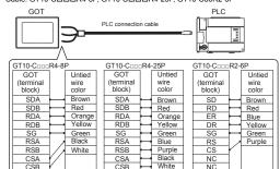
User-made cable is necessary, depending on the PLC. For the detail, refer to GOT2000 Series Connection Manual
