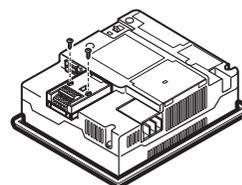
2) Fix the connection conversion adapter to the GOT using the provided M3 tapping screws. Tightening torque : 0.3 to 0.6 N·m
