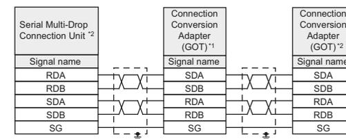
\*1 Set the terminating resistor selector to "OPEN".
