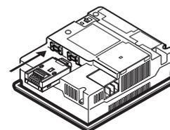
1) Connect the connection conversion adapter to the RS-422/485 interface on the GOT.
