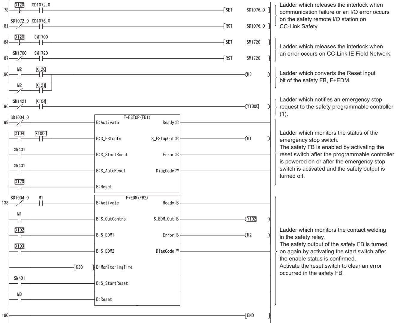
Figure 6.11 Safety FB program for safety programmable controller (2)
