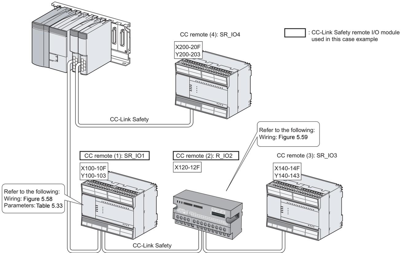
Figure 5.57 Safety device connection diagram
