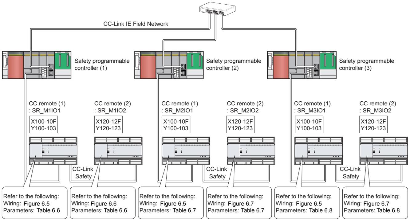
Figure 6.4 Safety device connection diagram
