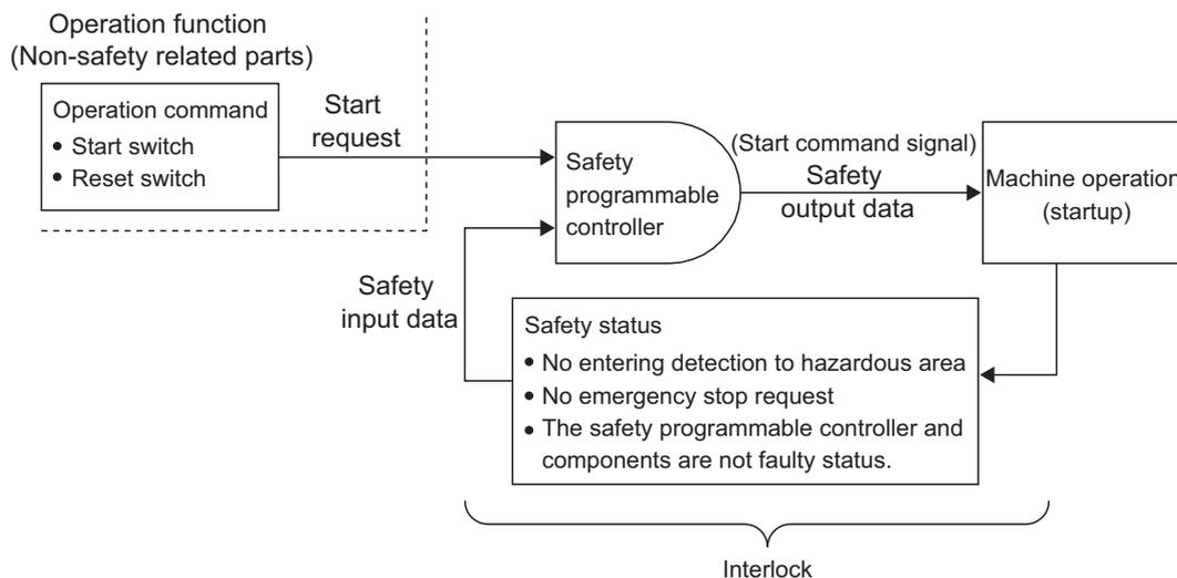
Figure 4.6 Configuration example of safety-related system
