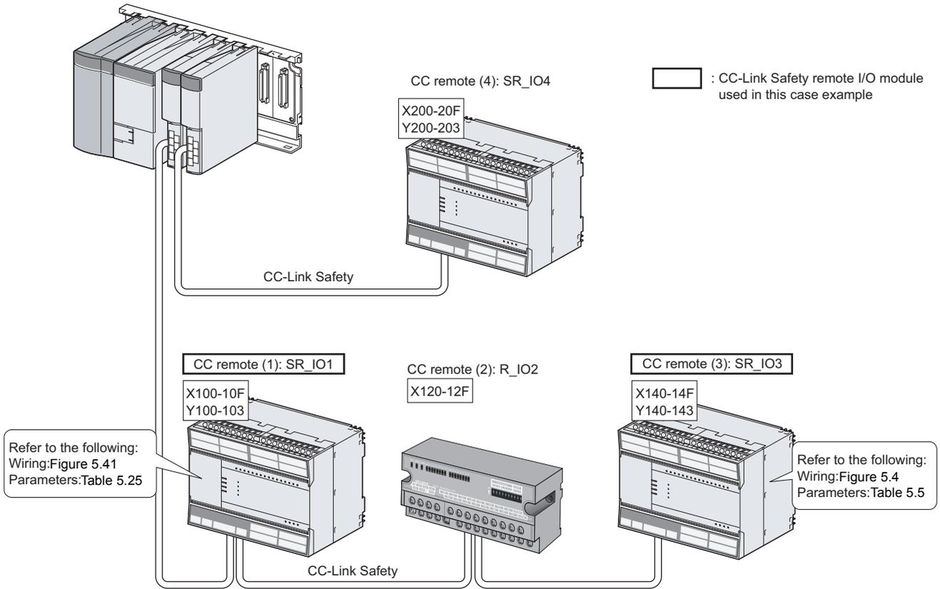
Figure 5.40 Safety device connection diagram
