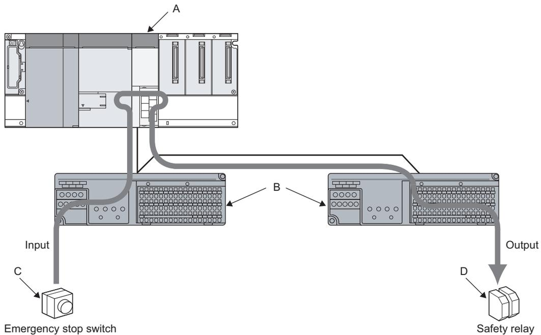
Figure 4.2 Example when one QS0J65BTS2-8D and one QS0J65BTS2-4T are used
