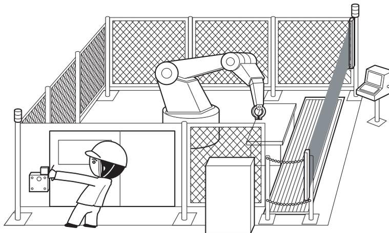
**Figure 5.39 Isolation of hazardous area by door interlock**
