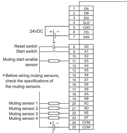
Figure 5.59 CC remote (2) R IO2 wiring
