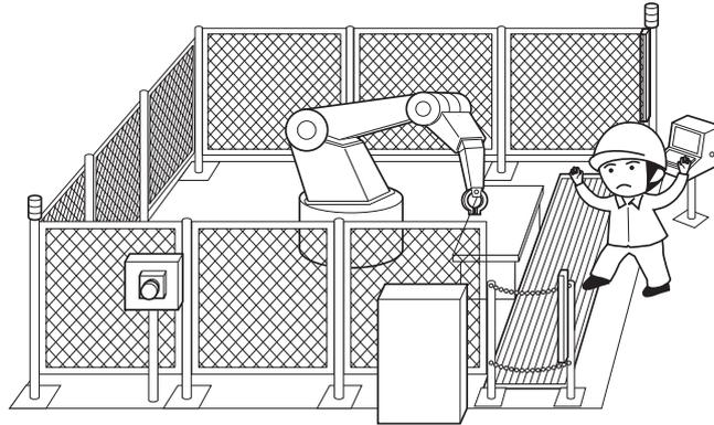
**Figure 5.32 Entering detection and existence detection**
