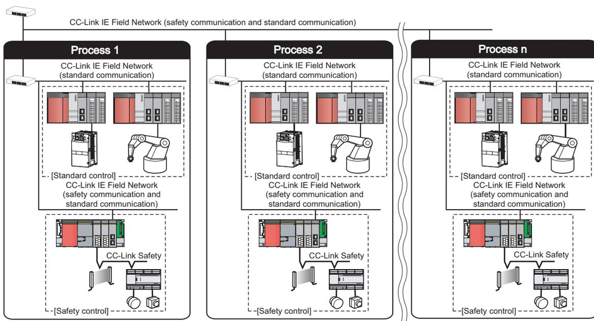
Figure 2.2 Safety control interfacing with control processes
