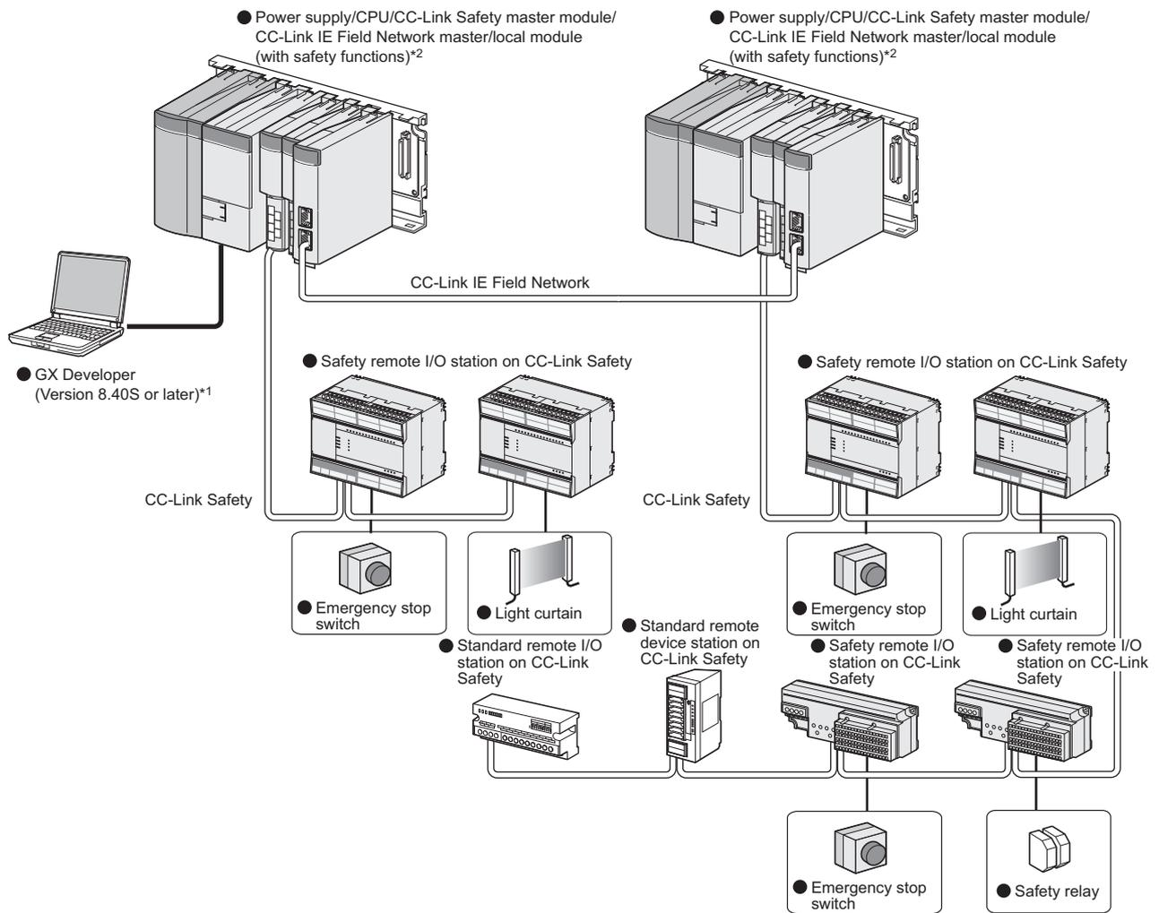
**Figure 1.1 System configuration of safety programmable controller**
