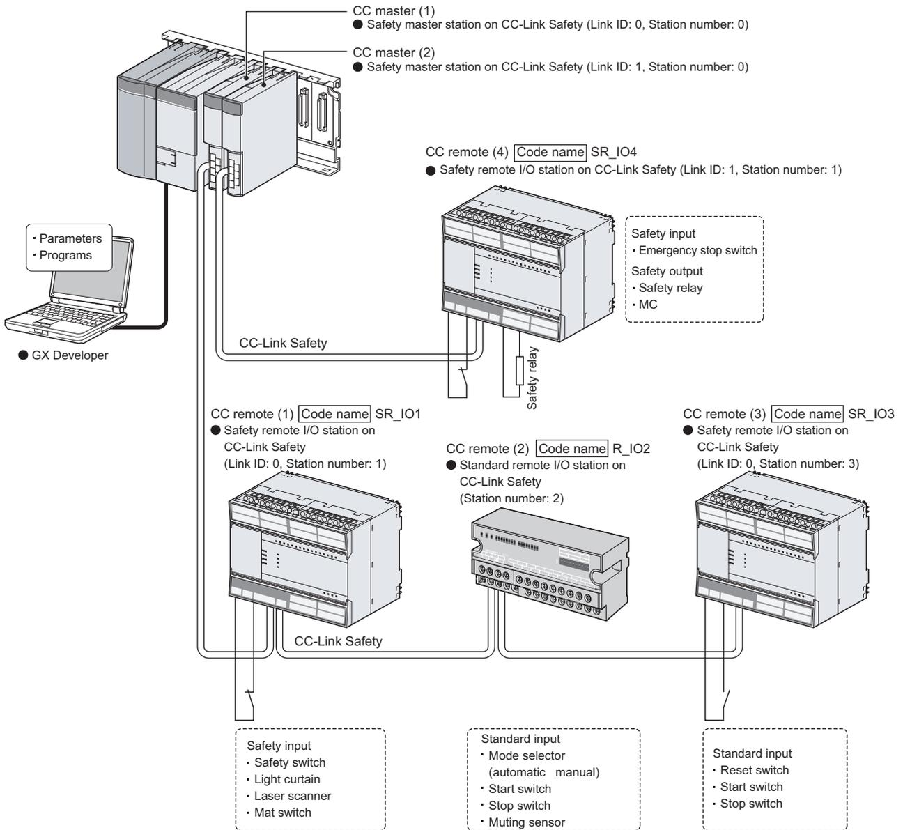
Figure 5.1 System configuration
