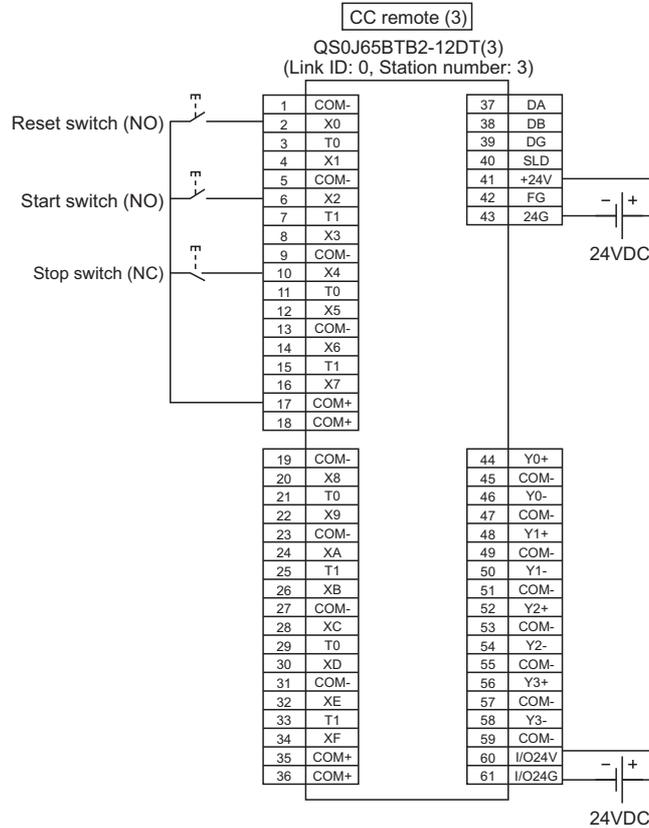
**Figure 5.4 CC remote (3) SR\_IO3 standard input wiring**
