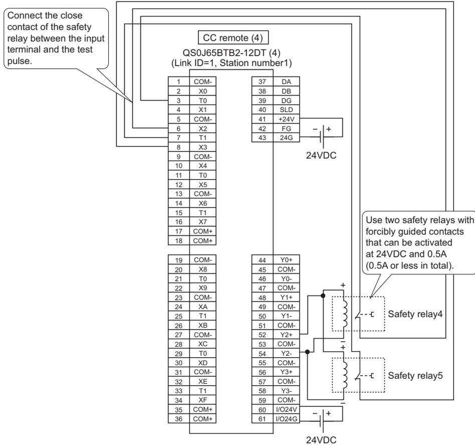
Figure 5.17 CC remote (4) SR\_IO4 wiring
