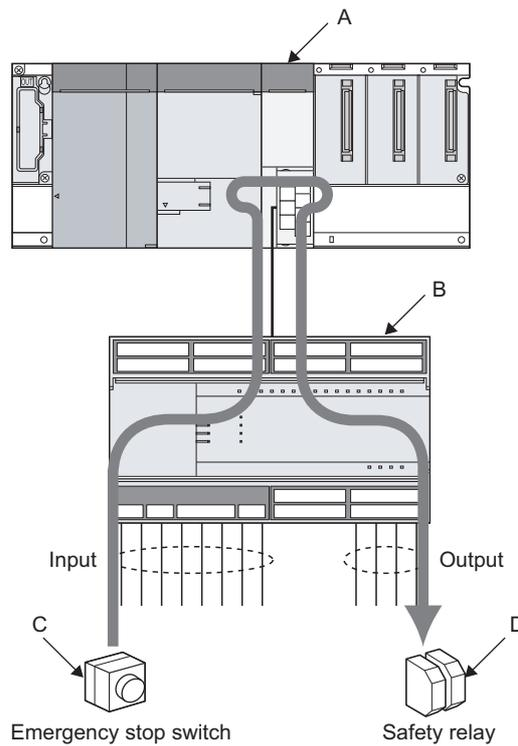
Figure 4.1 Example when one QS0J65BTB2-12DT is used
