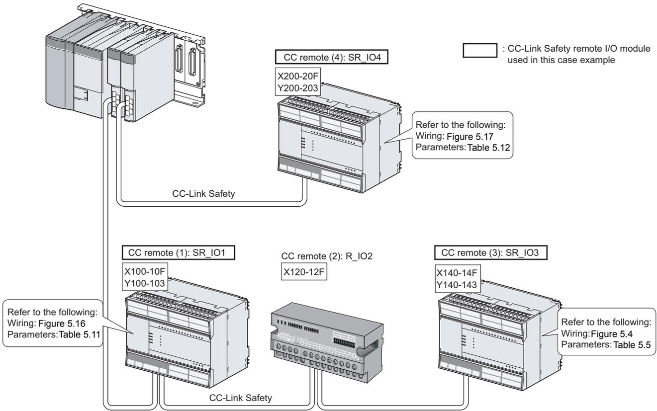
**Figure 5.15 Safety device connection diagram**
