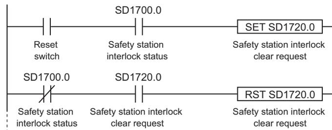
Figure 4.13 Example of the program that releases interlock of CC-Link IE Field Network during communication with any of station No. 1 to station No. 120
