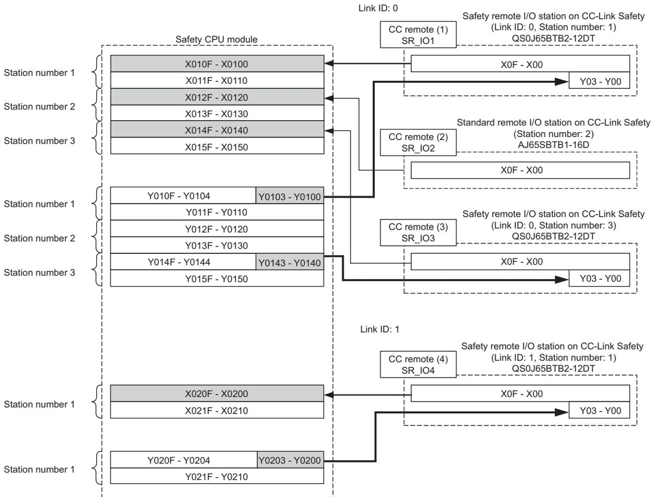
Figure 5.3 Relationship between safety CPU module devices and remote inputs/outputs
