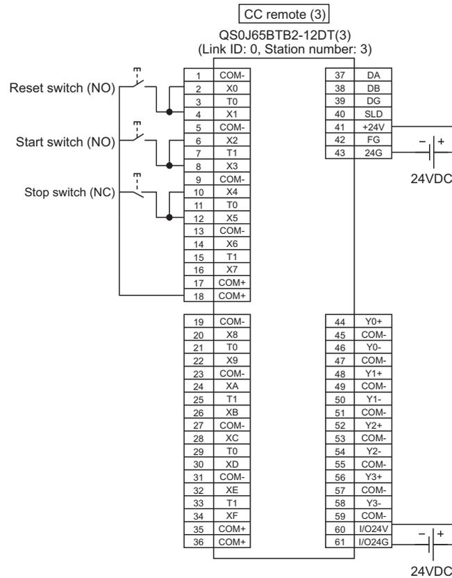
Figure 5.5 CC remote (3) SR\_IO3 standard input wiring
