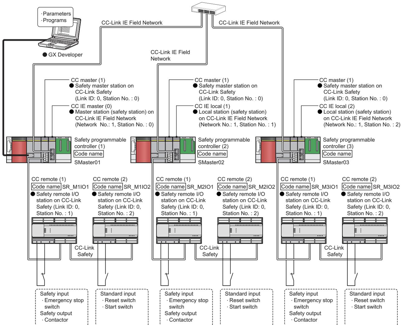
Figure 6.1 System configuration
