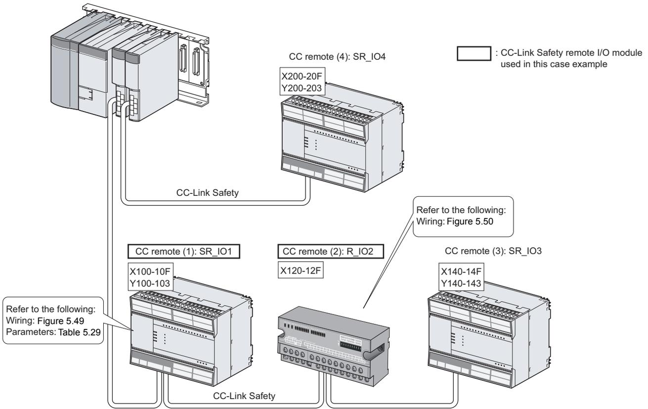
**Figure 5.48 Safety device connection diagram**
