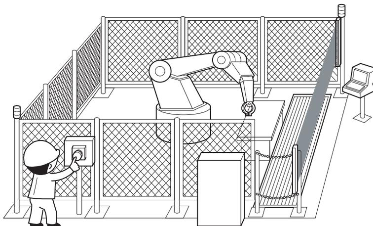
**Figure 5.6 Emergency stop switch**
