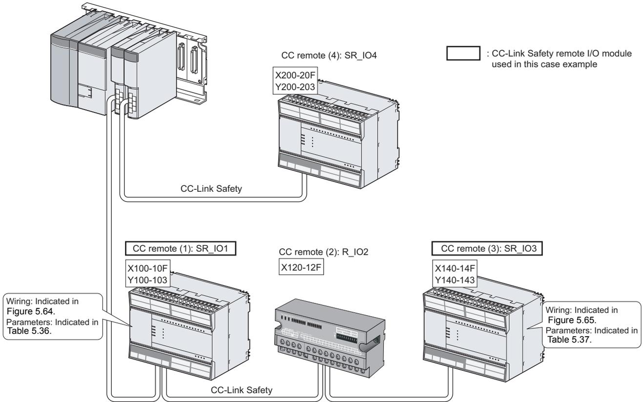
Figure 5.63 Safety device connection diagram
