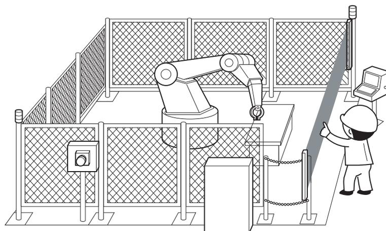
**Figure 5.23 Entering detection and existence detection circuit**
