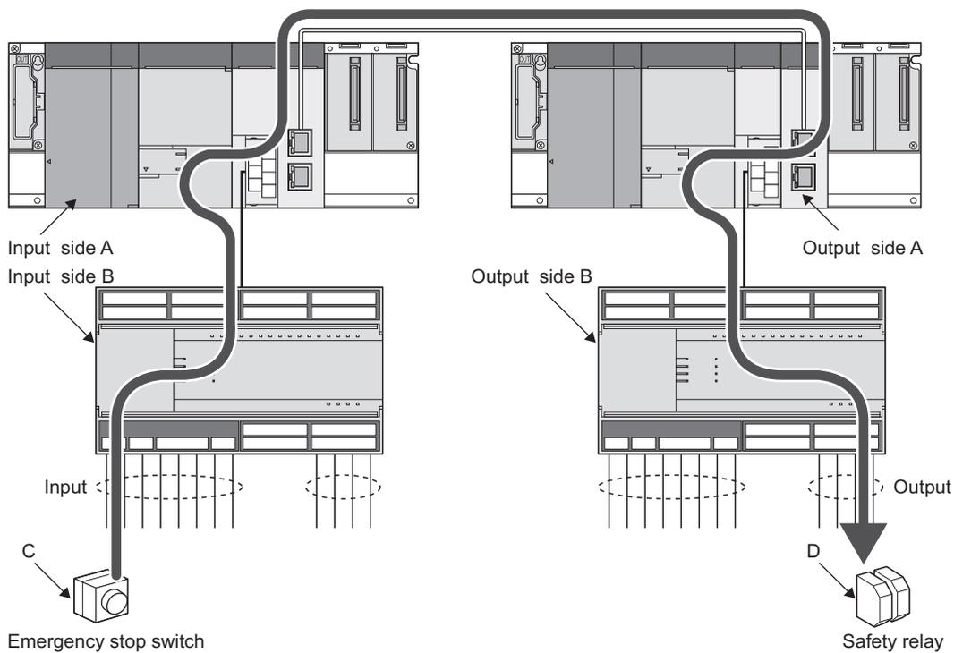
Figure 4.3 Example when CC-Link IE Field Network are used
