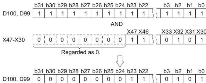
2 When three data are set ( $S_1 \wedge S_2 \rightarrow D$ ,  $(S_1 + 1, S_1) \wedge (S_2 + 1, S_2) \rightarrow (D + 1, D)$ )
