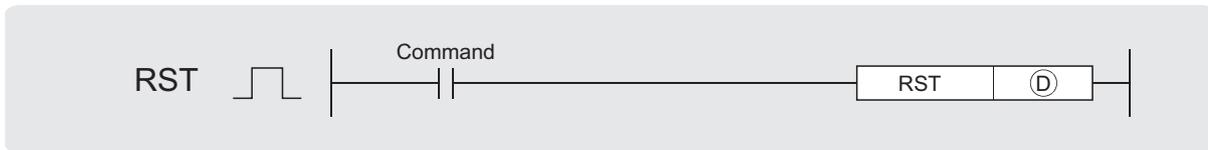
Ⓧ : Bit device number to be reset/ Word device bit designation (bits)
