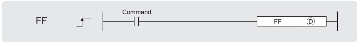
Ⓣ : Device number of the device to be reversed (bits)
