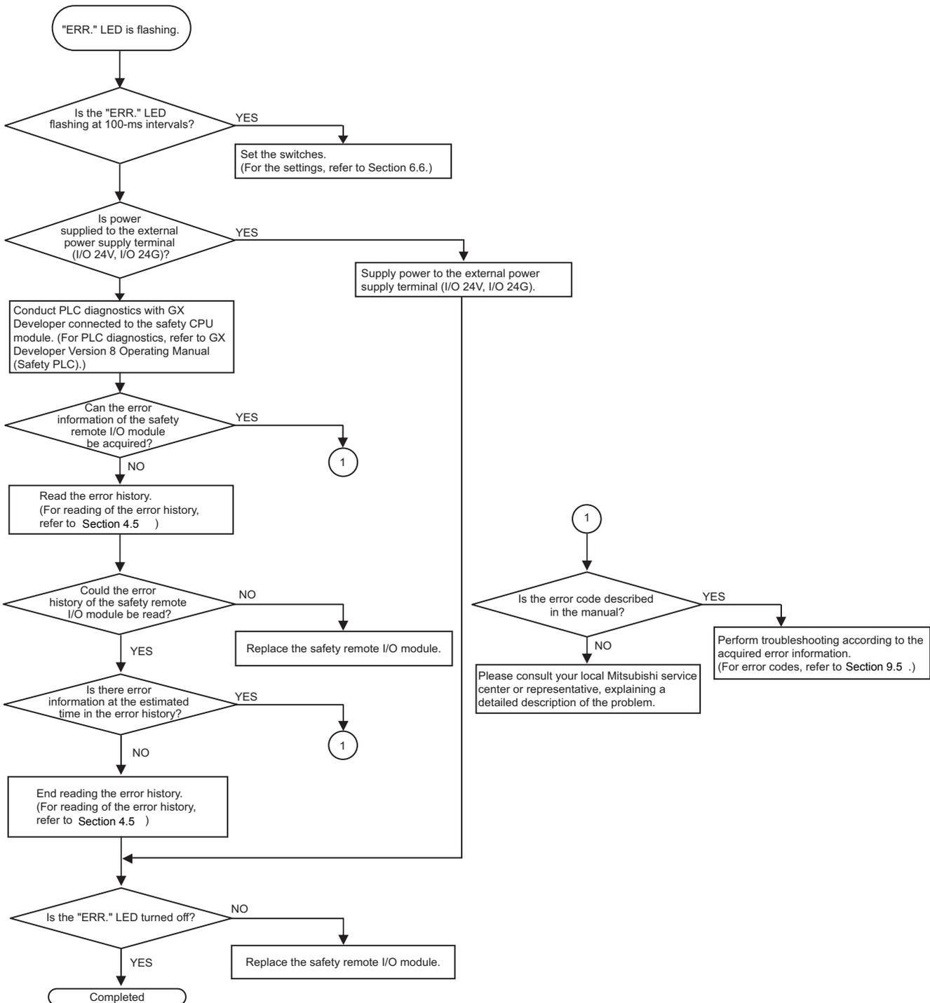
Figure 9.4 Flowchart for when the "ERR." LED flashes
