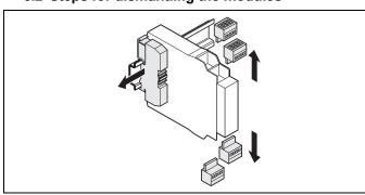
⇒ Remove the removable terminals with wiring and the end clips.
