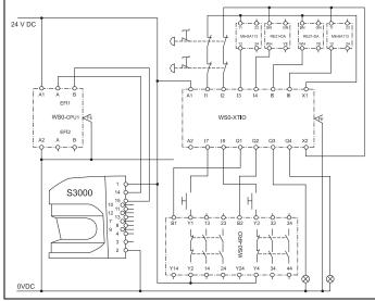
\*: The WS0-4RO cannot be used alone. The WS0-4RO performs the ON/OFF control via the WS0-XTIO.
