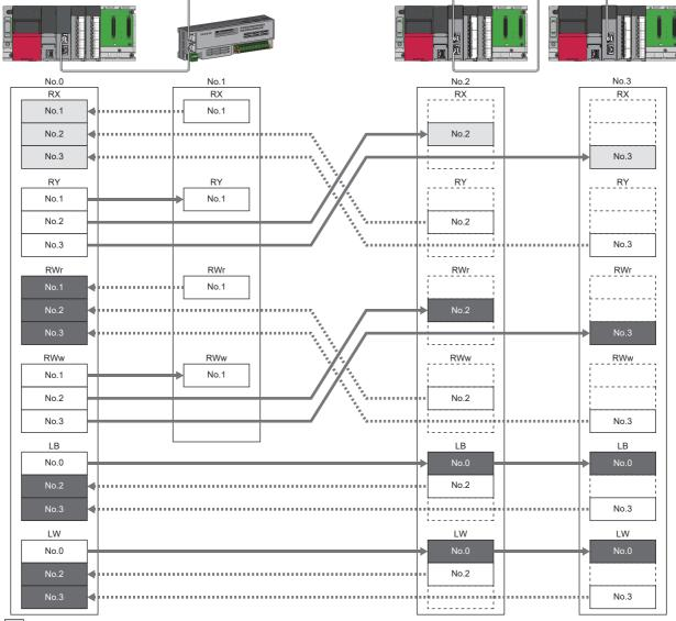
Devices that are held or cleared according to the parameter setting
