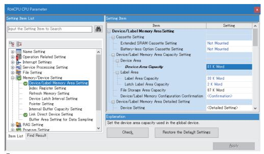
5. Set the values of "Points" of "Internal Relay M" and "Link Relay B" to 40K and the values of "Points" of "Data Register D" and "Link Register W" to 32K in the <Detailed Setting> window in "Device Setting".
