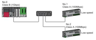
No.0: Master station (CC-Link IE TSN Plus module) No.1, No.2: Remote station Class A: CC-Link IE TSN Class A device Class B: CC-Link IE TSN Class B device
