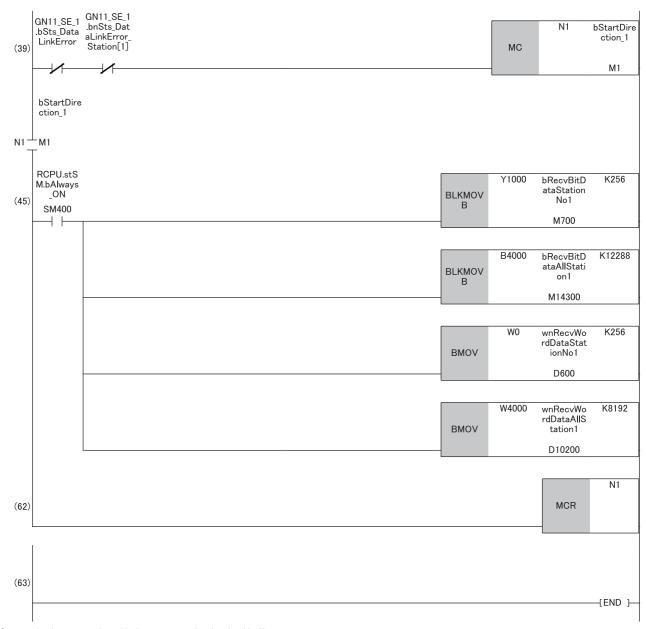
(4) Communication processing with the master station (station No.0)(45)Communication processing with a local station (station No.1)
