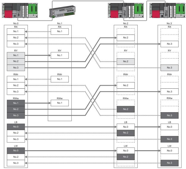
When the link refresh source is set to other than Y, data is held or cleared according to the parameter setting. When the link refresh source is set to Y, data is cleared regardless of the parameter setting.
