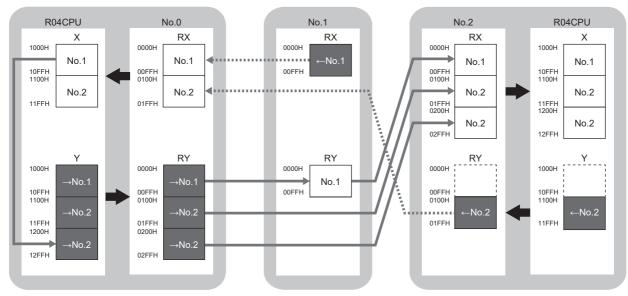
$\rightarrow$ No.1,  $\rightarrow$ No.2: Send range to station No.1, send range to station No.2  $\leftarrow$ No.1,  $\leftarrow$ No.2: Send range from station No.1, send range from station No.2
