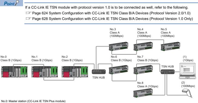
No.0: Master station (CC-Link IE TSN Plus module) No.1, No.2: Local station No.3 to No.8: Remote station (1), (2): Ethernet device Class A: CC-Link IE TSN Class A device Class B: CC-Link IE TSN Class B device
