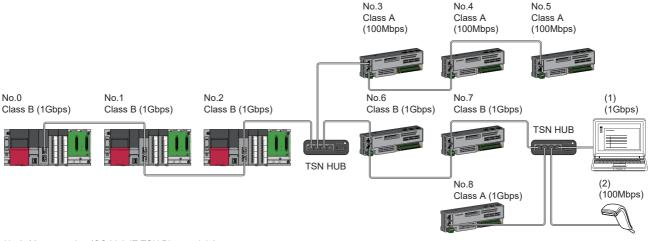
No.0: Master station (CC-Link IE TSN Plus module) No.1, No.2: Local station No.3 to No.8: Remote station (1), (2): Ethernet device Class A: CC-Link IE TSN Class A device Class B: CC-Link IE TSN Class B device
