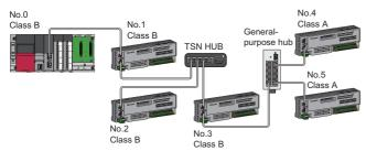
Connect the CC-Link IE TSN Class B device and CC-Link IE TSN Class A device via a TSN hub.
