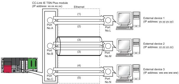
(1) Sending UDP data from CC-Link IE TSN Plus module's port number A to external device 1's port number L
