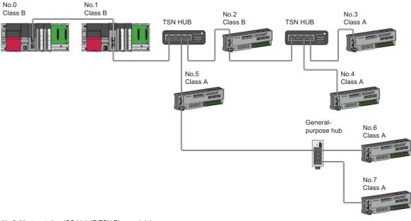
No.0: Master station (CC-Link IE TSN Plus module) No.1: Local station No.2 to No.7: Remote station Class A: CC-Link IE TSN Class A device Class B: CC-Link IE TSN Class B device
