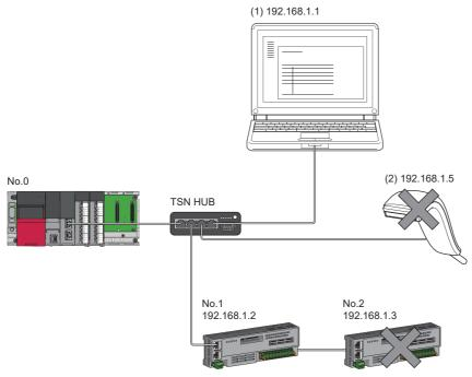
When the "Allow" IP addresses are set to 192.168.1.1 and 192.168.1.2 using the IP filter of the master station No.0: Only the Ethernet device (1) and device station No.1 can access the master station, and the Ethernet device (2) and device station No.2 cannot access the master station.
