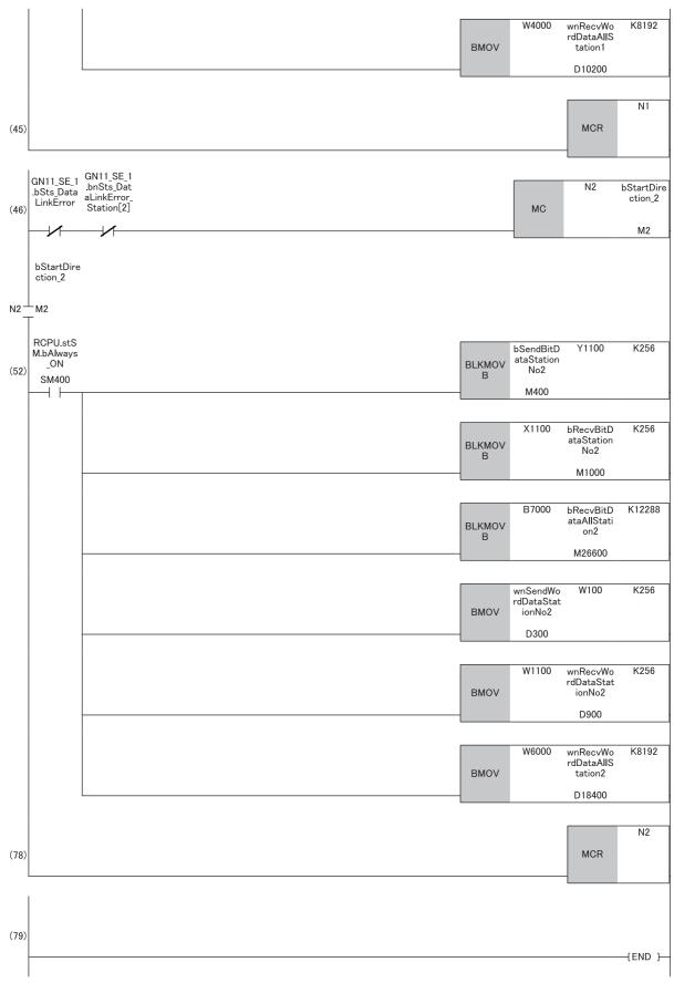
(4) Register the data that the own station will send to the local stations (station No.1 and station No.2).
