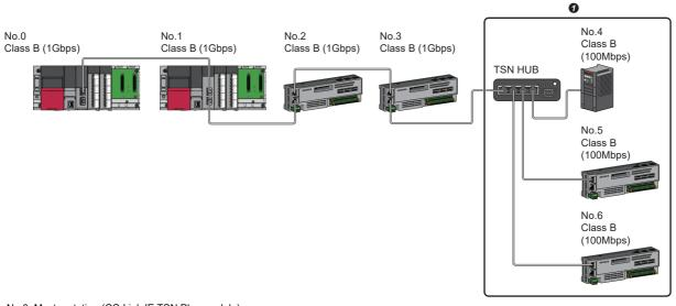
No.0: Master station (CC-Link IE TSN Plus module) No.1: Local station No.2 to No.6: Remote station Class A: CC-Link IE TSN Class A device Class B: CC-Link IE TSN Class B device Set the total cyclic data size within 2K bytes.
