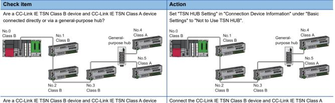
Are a CC-Link IE TSN Class B device and CC-Link IE TSN Class A device connected directly or via a general-purpose hub?
