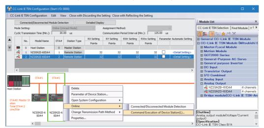
Select and right-click the device station, and select "Command Execution of Device Station" from "Online" to display the "Command Execution of Device Station" window.
