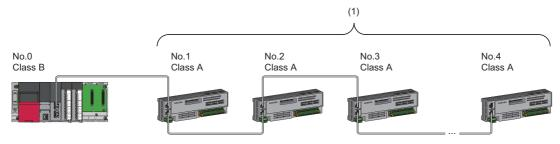
No.0: Master station (CC-Link IE TSN Plus module) No.1 to No.4: Remote station Class A: CC-Link IE TSN Class A device
