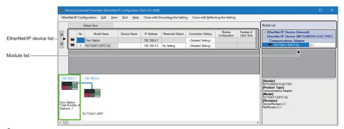
3. To detect and set the EtherNet/IP devices connected to the CC-Link IE TSN Plus module, click the [Detect Now] button. (SP Page 123 Automatic detection of EtherNet/IP devices)
