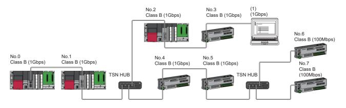
No.0: Master station (CC-Link IE TSN Plus module) No.1, No.2: Local station No.3 to No.7: Remote station (1) Ethernet device
