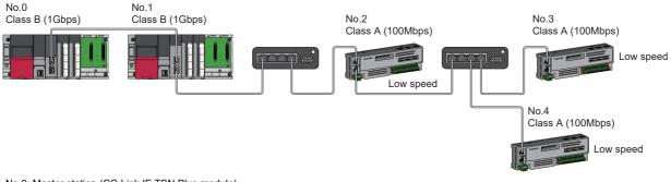
No.0: Master station (CC-Link IE TSN Plus module) No.1: Local station No.2, No.3, and No.4: Remote station Class A: CC-Link IE TSN Class A device Class B: CC-Link IE TSN Class B device
