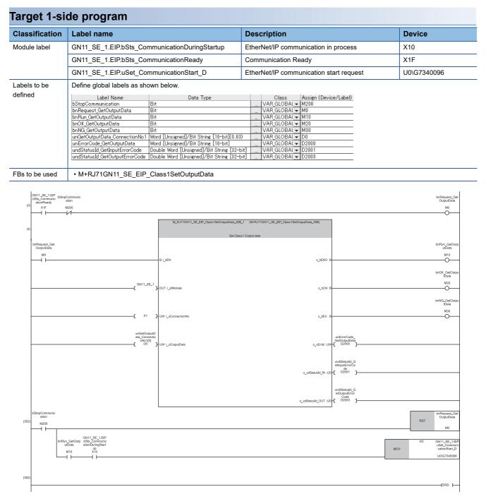
(0) Set the processing for output data to connection No.1 and start EtherNet/IP communication.
