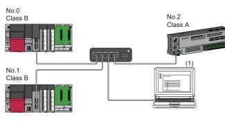
No.0: Master station (CC-Link IE TSN Plus module) No.1: Local station No.2: Remote station (1) Ethernet device Class A: CC-Link IE TSN Class A device Class B: CC-Link IE TSN Class B device
