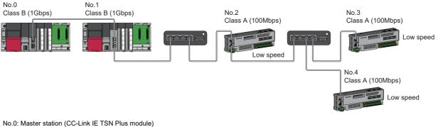
No.1: Local station No.2, No.3, and No.4: Remote station Class A: CC-Link IE TSN Class A device Class B: CC-Link IE TSN Class B device
