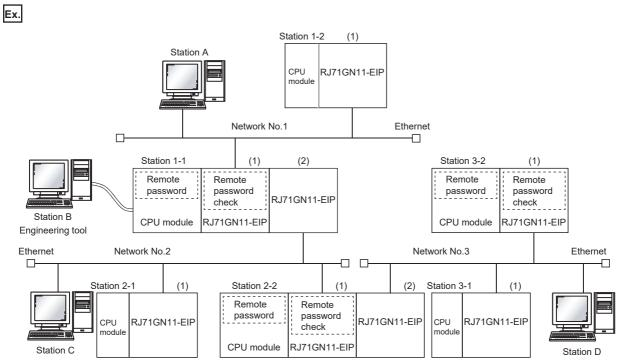
The password can be unlocked and locked by the following external devices.
