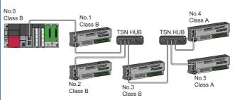
Do not allow the cyclic data size to exceed 2K bytes in total (1) for all device stations on the CC-Link IE TSN Class A device side at the boundary between CC-Link IE TSN Class B devices and CC-Link IE TSN Class A devices.
