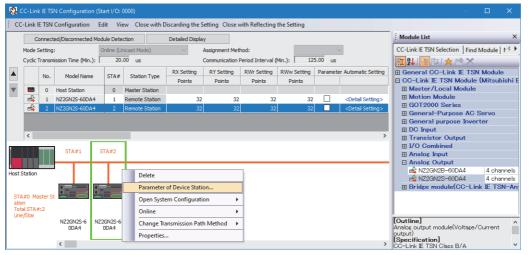
Select and right-click the device station, and select "Parameter of Device Station" to display the "Parameter of Device Station" window.
