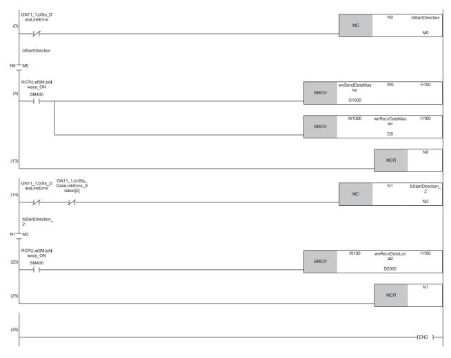
(4) Communication program with the master station (station No.0)(20)Communication program with a local station (station No.2)
