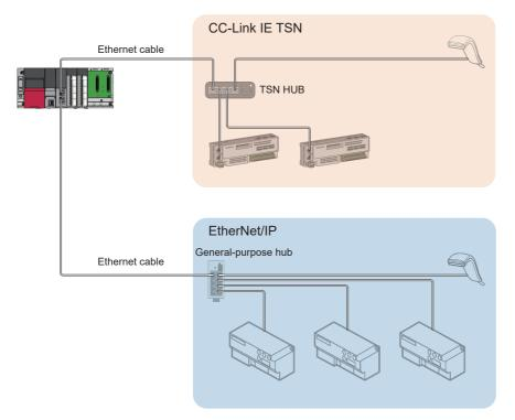
A single CC-Link IE TSN Plus module can communicate with CC-Link IE TSN and EtherNet/IP compatible products. While CC-Link IE TSN is used, EtherNet/IP compatible products can be used. Both networks can be used simultaneously without affecting the performance of each other.
