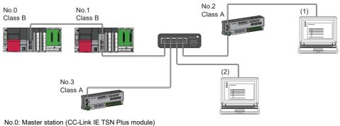
No.1: Local station No.2, No.3: Remote station (1), (2): Ethernet device Class A: CC-Link IE TSN Class A device Class B: CC-Link IE TSN Class B device
