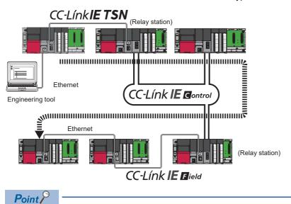
Communications can be made with stations up to eight networks apart (number of relay stations: 7).
