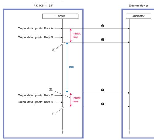
(1) If the output data is updated within the time set for "Inhibit Time" since the last transmission, the transmission will wait until the Inhibit time has elapsed.
