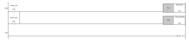
(0) The refresh processing of the module label is performed. (The processing is required when using the module function block.) When the refresh processing is completed, 'Refresh execution status' (M0) is turned on.
