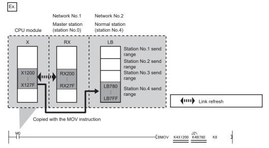
A link direct device cannot be specified for both the first and second arguments. Either one of them must use link refresh and specify the CPU device.
