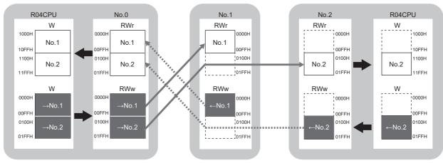
$\rightarrow$ No.1,  $\rightarrow$ No.2: Send range to station No.1, send range to station No.2  $\leftarrow$ No.1,  $\leftarrow$ No.2: Send range from station No.1, send range from station No.2
