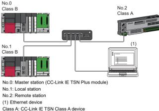
Class A: CC-Link IE TSN Class A device Class B: CC-Link IE TSN Class B device
