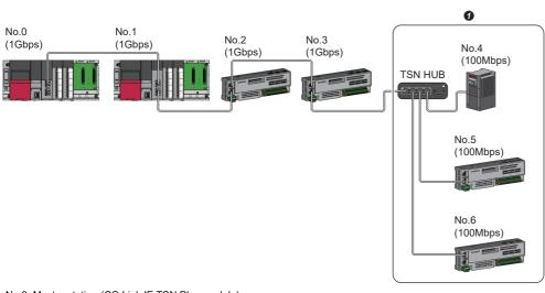
No.0: Master station (CC-Link IE TSN Plus module) No.1: Local station No.2 to No.6: Remote station Set the total cyclic data size within 2K bytes.
