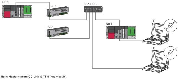
No.0: Master station (CC-Link IE TSN Plus module) No.1: Local station No.2, No.3: Remote station (1) CC-Link IE TSN Communication Software
