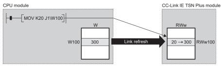
• Good example (Directly accessing the link device as well as writing the same data to the device of the CPU module)
