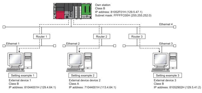
Ex. When the network addresses differ between the CC-Link IE TSN Plus module on the own station and the external device
