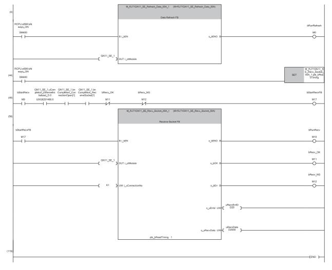
(0) The refresh processing of the module label is performed. (The processing is required when using the module function block.) When the refresh processing is completed, M0 is turned on.
