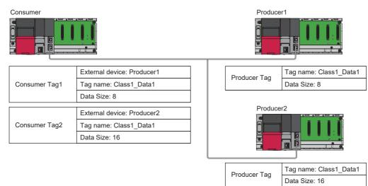
• When the data size of Producer Tag is different from the data size of Consumer Tag, Producer may send an error response to Consumer.
