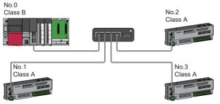
No.0: Master station (CC-Link IE TSN Plus module) No.1, No.2, and No.3: Remote station Class A: CC-Link IE TSN Class A device Class B: CC-Link IE TSN Class B device
