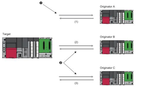
(1) Originator A and the target are connected via connection No.1 (Exclusive Owner (Class1 instance communications)).
