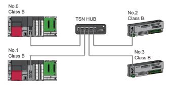
No.0: Master station (CC-Link IE TSN Plus module) No.1: Local station No.2, No.3: Remote station Class B: CC-Link IE TSN Class B device • When connecting a CC-Link IE TSN Class A device to a CC-Link IE TSN Class B device or connecting a CC-Link IE TSN Class A device in a star topology, connect them via a switching hub.
