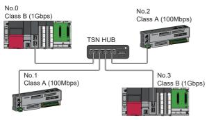
No.0: Master station (CC-Link IE TSN Plus module) No.1, No.2: Remote station No.3: Local station Class A: CC-Link IE TSN Class A device
