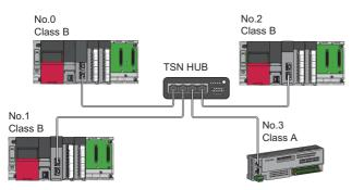
No.0: Master station (CC-Link IE TSN Plus module) No.1, No.2: Local station No.3: Remote station Class A: CC-Link IE TSN Class A device Class B: CC-Link IE TSN Class B device
