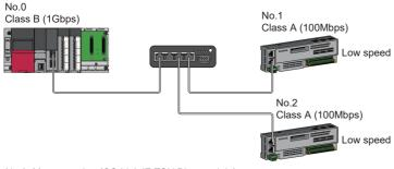
No.0: Master station (CC-Link IE TSN Plus module) No.1, No.2: Remote station Class A: CC-Link IE TSN Class A device
