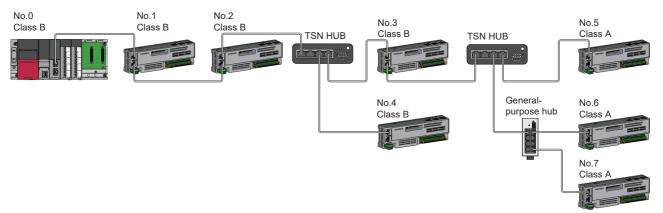
No.0: Master station (CC-Link IE TSN Plus module) No.1 to No.7: Remote station Class A: CC-Link IE TSN Class A device Class B: CC-Link IE TSN Class B device
