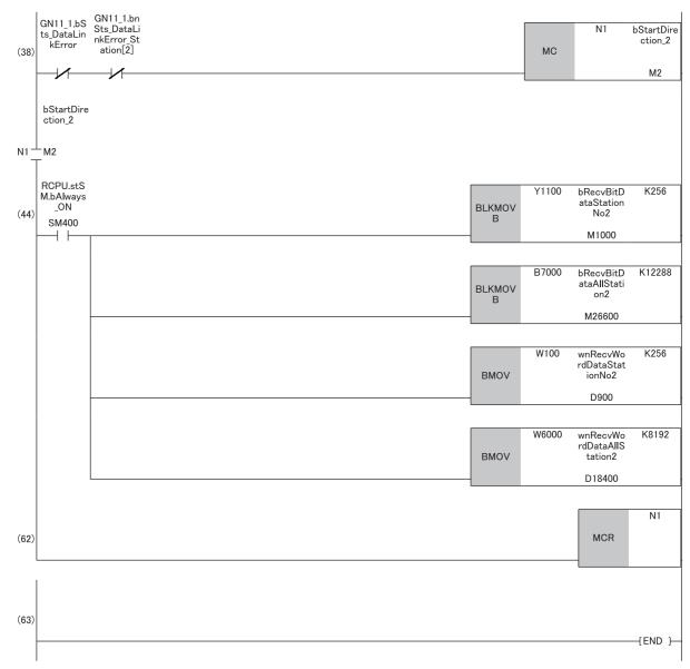
(4) Communication processing with the master station (station No.0)(44)Communication processing with a local station (station No.2)
