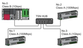
No.0: Master station (CC-Link IE TSN Plus module) No.1, No.2, and No.3: Remote station Class A: CC-Link IE TSN Class A device Class B: CC-Link IE TSN Class B device
