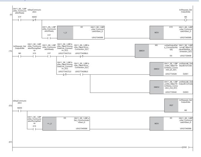
(0) Set the processing for output data to connection No.1 and start EtherNet/IP communication.
