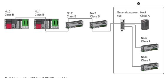
No.0: Master station (CC-Link IE TSN Plus module) No.1: Local station No.2 to No.6: Remote station Class A: CC-Link IE TSN Class A device Class B: CC-Link IE TSN Class B device Set the total cyclic data size within 2K bytes.
