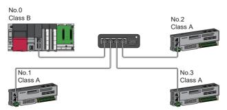
No.0: Master station (CC-Link IE TSN Plus module) No.1, No.2, and No.3: Remote station Class A: CC-Link IE TSN Class A device Class B: CC-Link IE TSN Class B device
