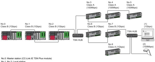
No.0: Master station (CC-Link IE TSN Plus module No.1, No.2: Local station No.3 to No.8: Remote station (1), (2): Ethernet device Class A: CC-Link IE TSN Class A device Class B: CC-Link IE TSN Class B device
