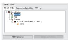
9. Select "Connection (Adapter Instance Communications)" in "Select Connection to be Added:" and click the [OK] button.
