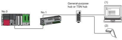
No.0: Master station (CC-Link IE TSN Plus module) No.1: Remote station (1), (2): Ethernet device
