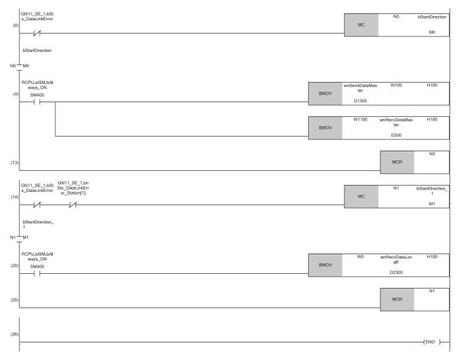
(4) Communication program with the master station (station No.0)(20)Communication program with a local station (station No.1)
