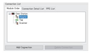
7. Select "Connection (Adapter Instance Communications)" in "Select Connection to be Added:" and click the [OK] button.
