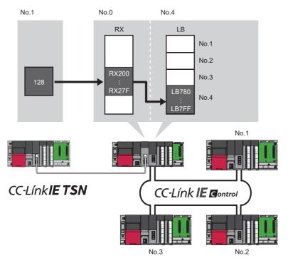
**1.** Select "0000: RJ71GN11-EIP (T+E) (Master Station) [RX/RWr]" for "Transfer Source Module" and "0020: RJ71GP21-SX (Normal Station)" for "Transfer Destination Module", and enter the transfer ranges of link devices.
