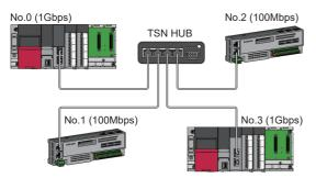
No.0: Master station (CC-Link IE TSN Plus module) No.1, No.2: Remote station No.3: Local station
