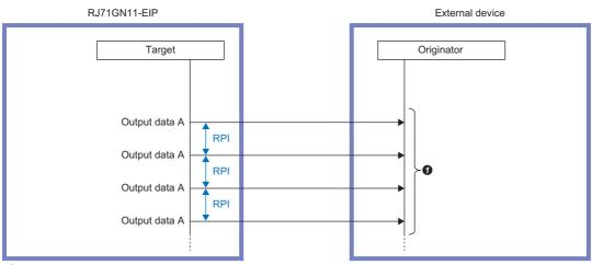
**1** Output data stored at the target side is automatically sent at RPI intervals.
