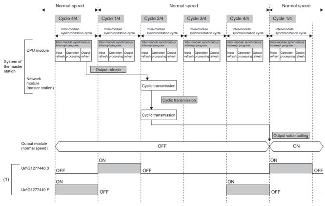
(1) The communication cycle timing can be checked with the 'Communication cycle timing' (Un\G1277440 to Un\G1277441) of the buffer memory. The timing of data refreshed in the CPU module can also be checked with this buffer memory area. The 0th bit in this buffer memory area is turned on during the first (1/4) cycle for normal speed. In addition, the 15th bit in this buffer memory area is turned on during the last (4/4) cycle for normal speed. (SP Page 540 Communication cycle timing)
