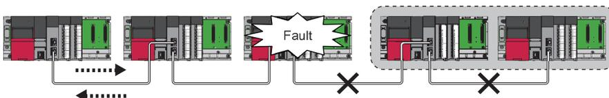
Stations connected after the faulty station are disconnected.
