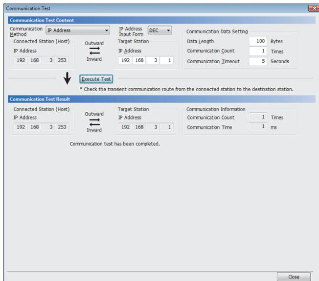
1. Display the "Communication Test" window and select "Network No./Station No." or "IP Address" from "Communication Method".
