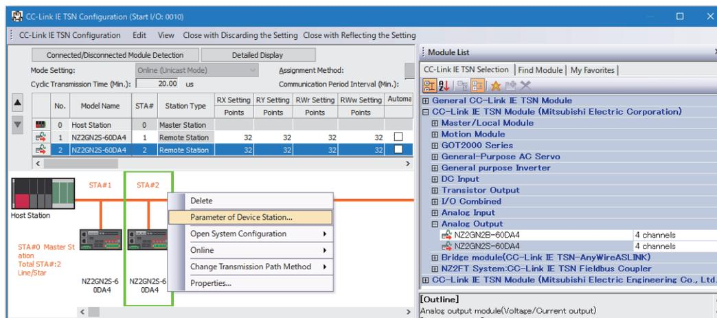
Select and right-click the device station, and select "Parameter of Device Station" to display the "Parameter of Device Station" window.
