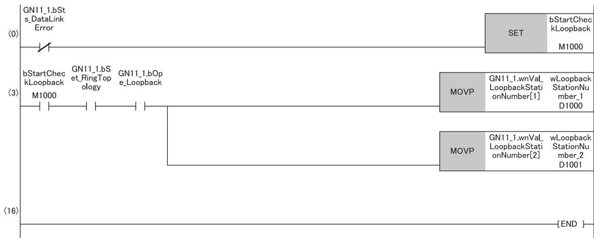
(3) When 'Network topology setting' (SB0078) and 'Loopback status' (SB0065) are on, 'Loopback station number 1' (SW0070) and 'Loopback station number 2' (SW0071) are saved.
