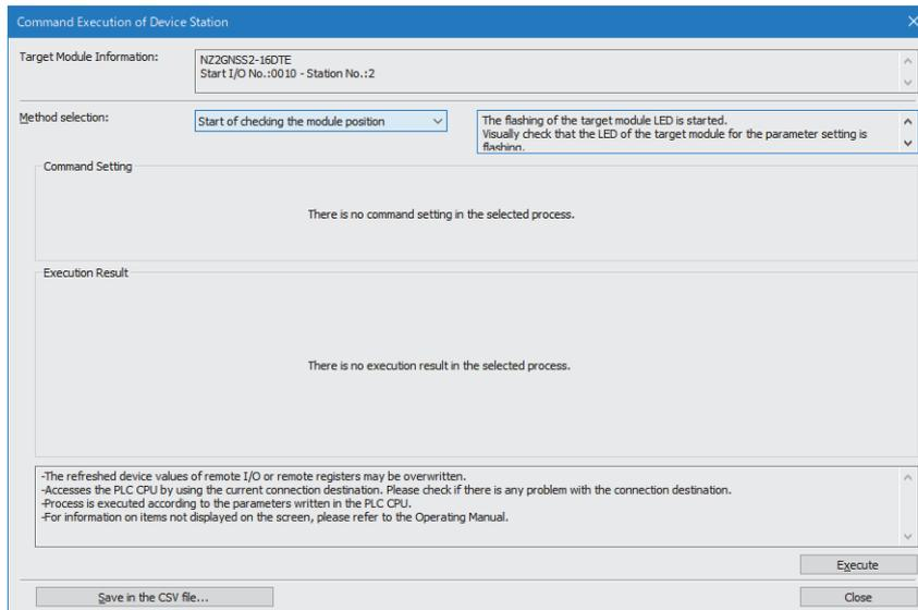
5. The SAFETY LED of the NZ2GNSS2-16DTE flashes. Check if the NZ2GNSS2-16DTE on which the SAFETY LED flashes has been installed on the desired position.
