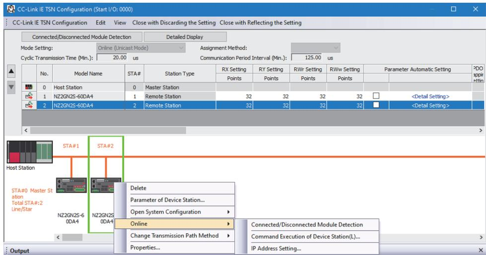
Select and right-click the device station, and select "Command Execution of Device Station" from "Online" to display the "Command Execution of Device Station" window.
