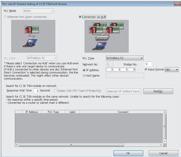
5. Double-click the icon set in step 4, and open the "PLC side I/F Detailed Setting of CC IE TSN/Field Module" window.
