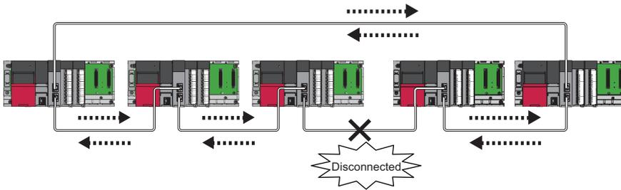
Even if a cable disconnection occurs, the system automatically performs a loopback to continue the data link.
