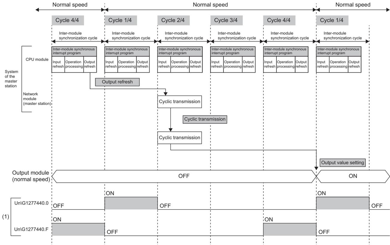
(1) The communication cycle timing can be checked with 'Communication cycle timing' (UnG1277440 to UnG1277441) of the buffer memory. The timing of data refreshed in the CPU module can also be checked with this buffer memory area. The 0th bit in this buffer memory area is turned on during the first (1/4) cycle for normal speed. In addition, the 15th bit in this buffer memory area is turned on during the last (4/4) cycle for normal speed. (Page 288 Communication cycle timing (RJ71GN11-T2 only))
