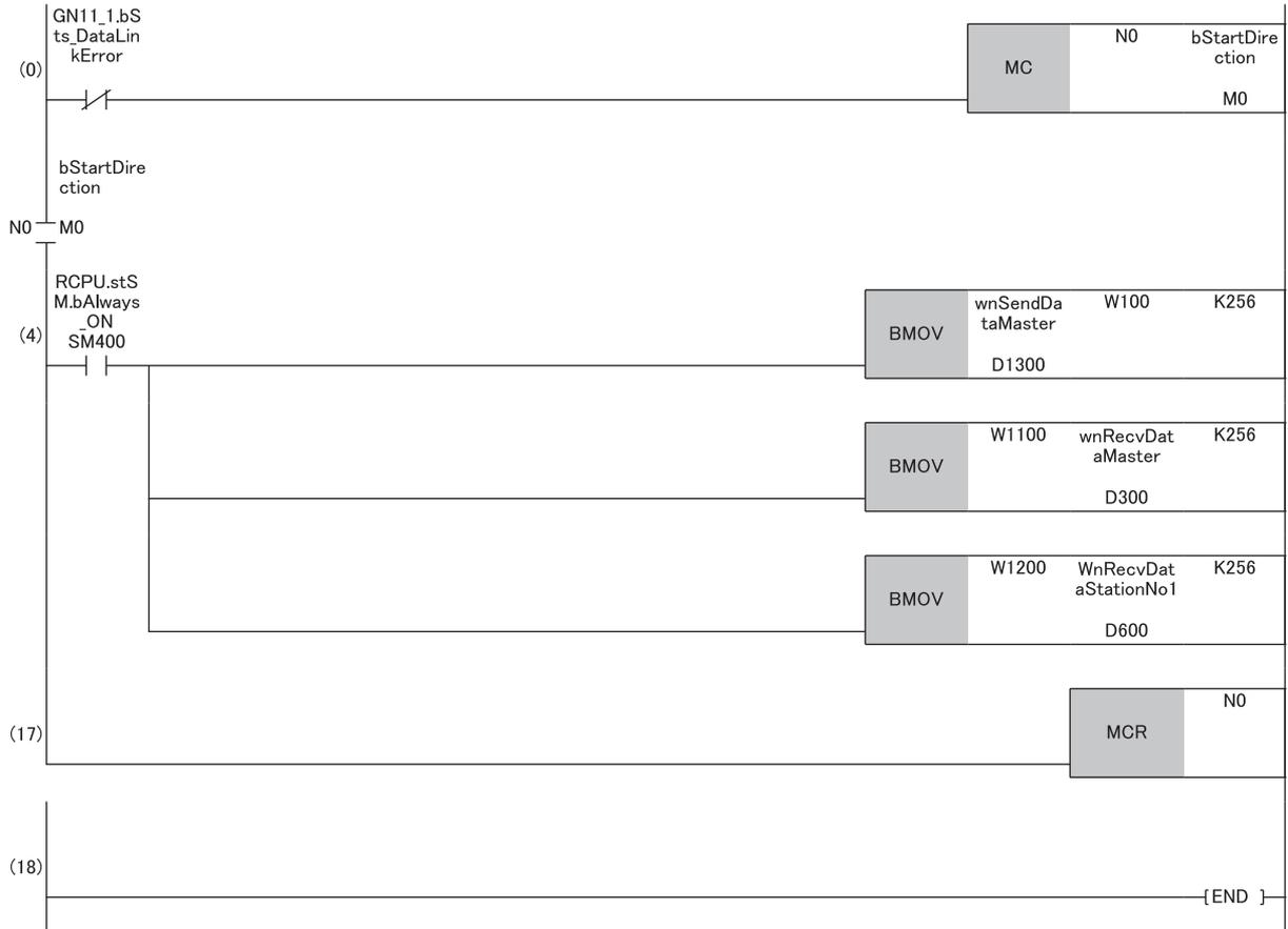
(4) Communication program with the master station (station No.0) and a remote station (station No.1)
