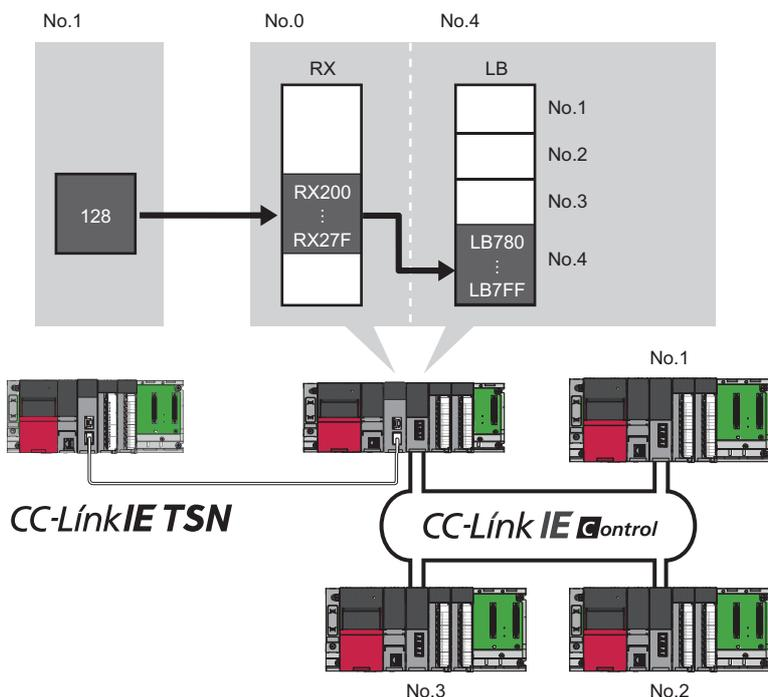
1. Select "0000: RJ71GN11-T2 (Master Station) [RX/RWr]" for "Transfer Source Module" and "0020: RJ71GP21-SX (Normal Station)" for "Transfer Destination Module", and enter the transfer ranges of link devices.
