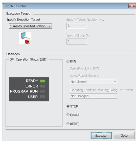
1. Select the module where the remote operations are performed in the "CC-Link IE TSN/CC-Link IE Field Diagnostics" window.
