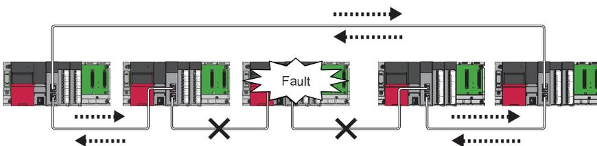
The system disconnects faulty stations and automatically performs a loopback to continue the data link.
