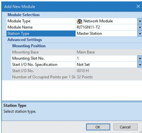
10. Click the [OK] button to use the module labels of the safety function module.
