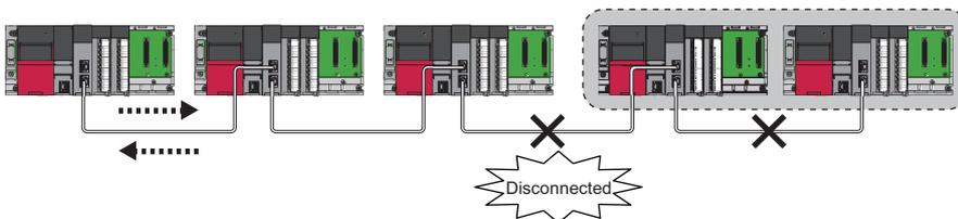
Stations connected after the cable disconnection point are disconnected.
