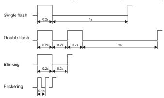
\*2 The CAN RUN LED and CAN ERR LED alternately flash while the LSS services are in progress.
