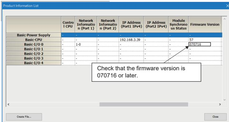
2. If not, upgrade the version of the basic system software, boot software, and network boot software.\*1
