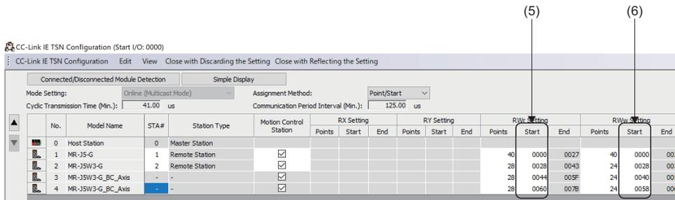
If the communication mode is unicast and a local station does not exist in the network configuration settings, the Motion module will ignore the setting of the motion control station link device start.
