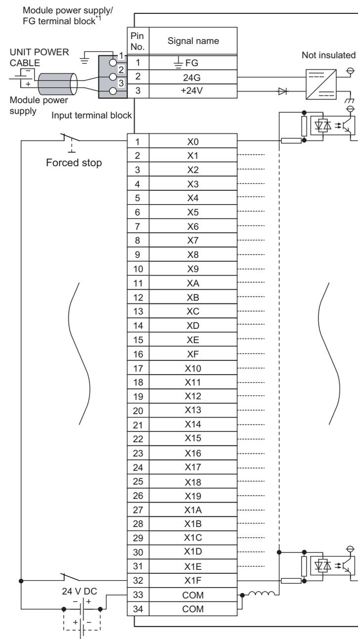
\*1 Only one wire can be connected to a terminal of the terminal block for module power supply and FG. Multiple wires cannot be connected to a terminal. Connecting two or more wires may cause a poor contact.
