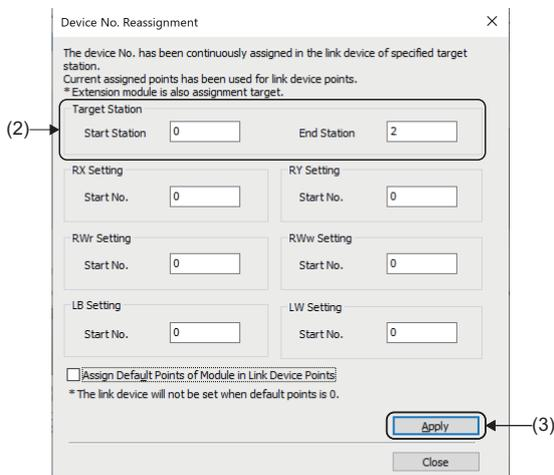
When reallocating device numbers, if the station code of the standard station is included in the setting range, the device setting of the standard station will be overwritten. If a standard station is set, set the station number of the standard station to outside of the setting range, or manually set the motion control station link device start/end.
