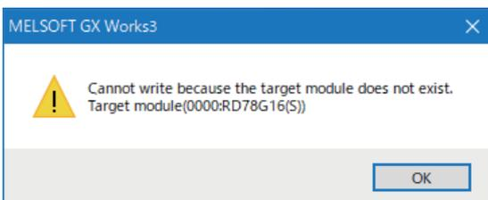
When the data of the CPU module is deleted, or the module parameter of RD78G\_ is written, the module model name is set to "RD78G\_" (PLCopen motion control FB mode).
