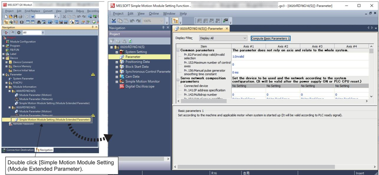
Double click [Simple Motion Module Setting (Module Extended Parameter)].
