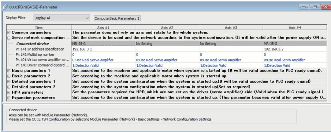
2. Set the axis 4 as the servo input axis in the "Input Axis Parameter" window.
