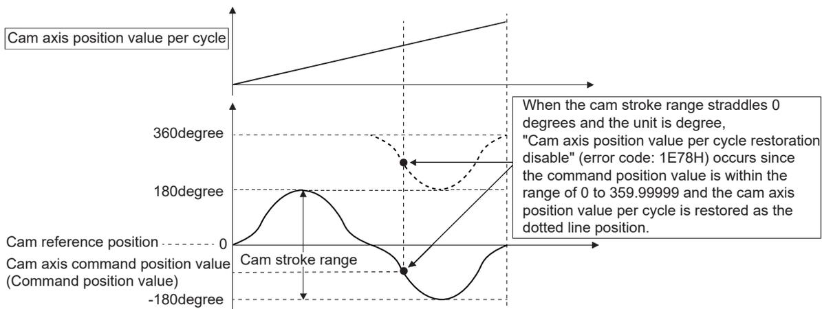
Restore the position value within the cam stroke range of 0 to less than 360[degree].
