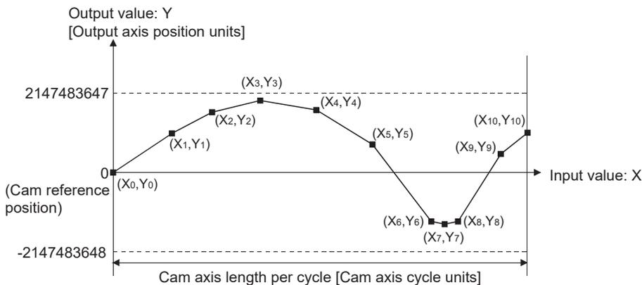
When an input value that is 0 or the cam axis length per cycle does not exist in the coordinate data, the coordinate is calculated from the line segment between the nearest two coordinates.
