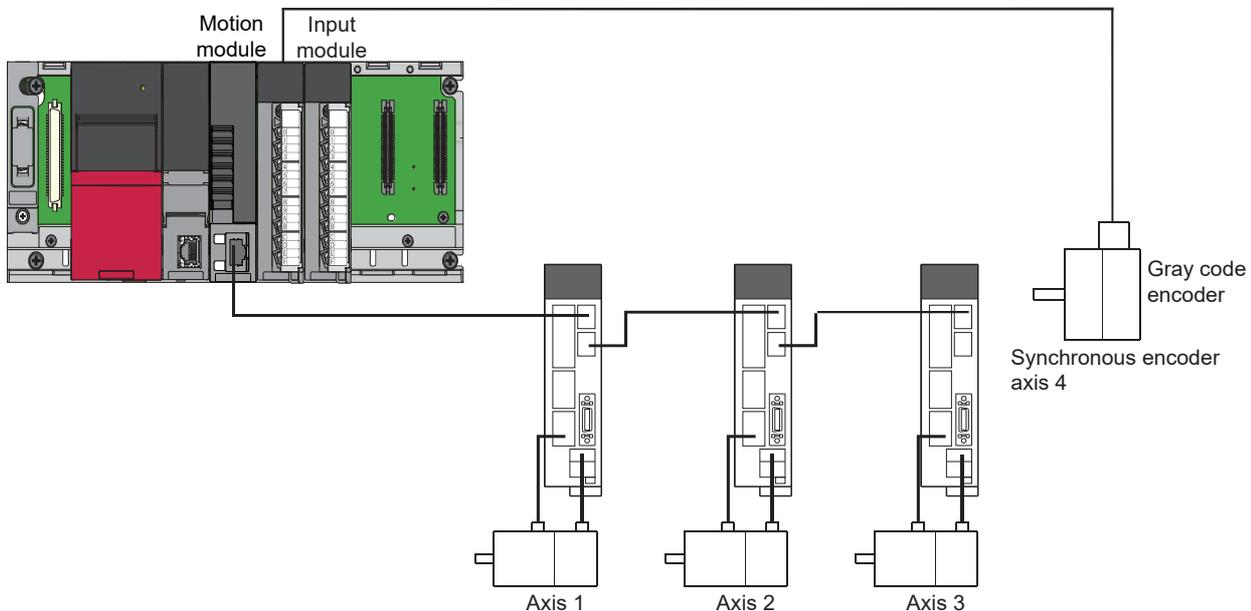
Set "201: Synchronous encoder via CPU" in "[Pr.320] Synchronous encoder axis type" of synchronous encoder axis 4.
