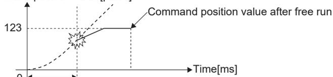
Forced stop occurred during operation, and the cam decelerates to a stop. (Advanced synchronous control mode is cancelled.)
