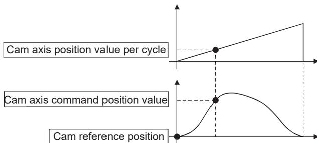
Select from 3 objects as follows in "[Pr.462] Cam axis position restoration object" which position is to be restored. (Refer to [Page 147](#) Cam Axis Position Restoration Method for details on the restoration method.)
