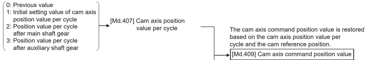
[Pr.463] Setting method of cam reference position
