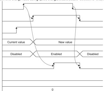
When "Cd.12: Acceleration/deceleration time change value during speed change, enable/disable" selection is "disabled"
