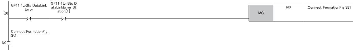
(0) Checks the data link status of the remote head module (station number 1).
