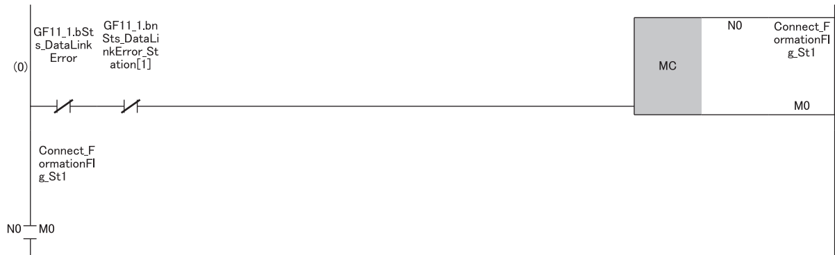
(0) Checks the data link status of the remote head module (station number 1).
