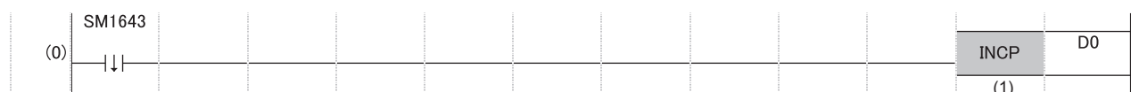
(1) The instruction will be executed in the second scan after the system switching.
