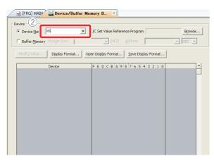
The values of devices and the ON/OFF status of contacts/coils are displayed.
