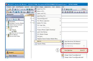
The values of devices and the ON/OFF status of contacts/coils are displayed.
