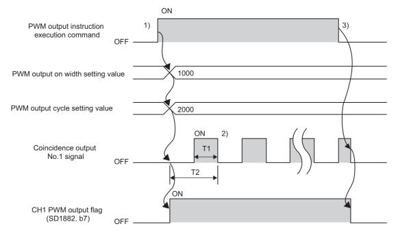
T1: PWM output on width setting value T2: PWM output cycle setting value
