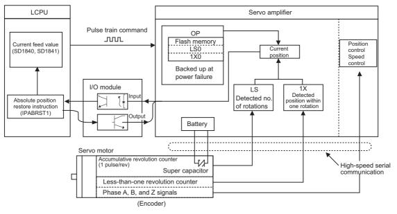
\*1 Operation to output a deviation counter clear signal to the servo amplifier at the OP position. This operation must be performed before absolute position restoration. When other than Count 2 is selected: Perform machine OPR, output a deviation counter clear signal. When Count 2 is selected: Wire a general-purpose output signal to the deviation counter clear signal line of the servo amplifier, perform JOG operation to adjust the position, and then turn the signal on.
