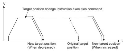
• If the position of the workpiece upon establishment of the execution command for Target position change instruction (IPTPCHG1(P)) exceeds the position at which to start decelerating to the new target value over the deceleration stop time, the axis decelerates to a stop and then positions itself to the new target position.
