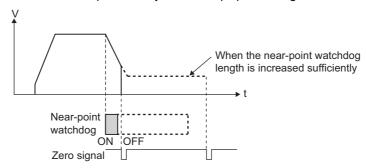
For the method to calculate the distance from the near-point dog ON position to OP, refer to Page 69, Section 7.6 (8).
