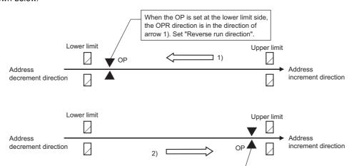
When the OP is set at the upper limit side, the OPR direction is in direction of arrow 2). Set "Forward run direction".
