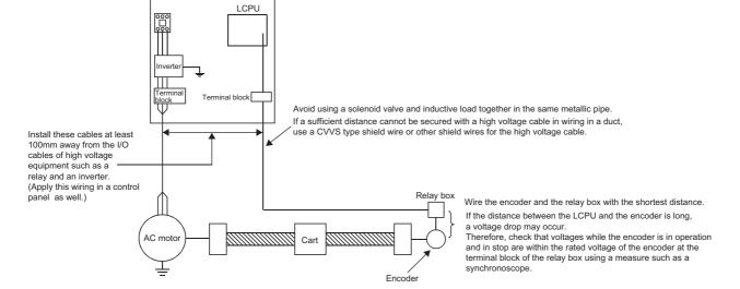
• Ground the shielded twisted pair cable on the encoder side (relay box). (This example shows wiring using 24V sink type.)
