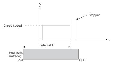
When starting position of the machine OPR is in interval B (between the near-point dog OFF position and stopper) in the figure below, no near-point dog is detected and thus the axis may collide with the stopper at the OPR speed. Make sure the near-point dog is longer than the distance to the stopper.
