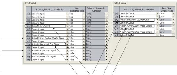
Select an option from the pull-down menu as necessary. According to the settings, external signals are assigned.
