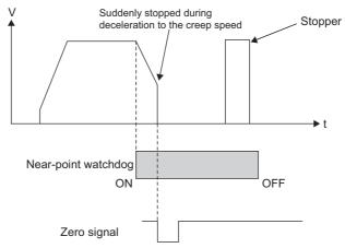
Do not input a zero signal before machine OPR is started. If a zero signal is already input externally when machine OPR is started, a "Zero signal ON" error (Axis 1 error code: 1200) occurs and machine OPR is not performed.
