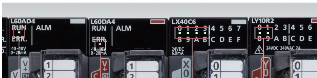
LEDs are located on the top front surface of the modules.
