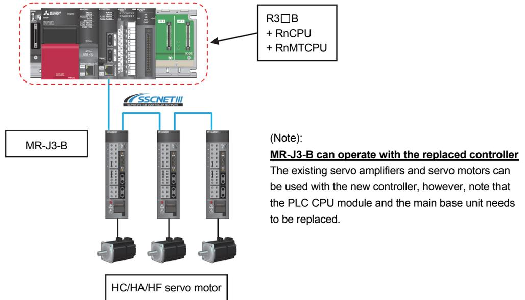
(2) When the MR-J3-B servo amplifier has malfunctioned.
