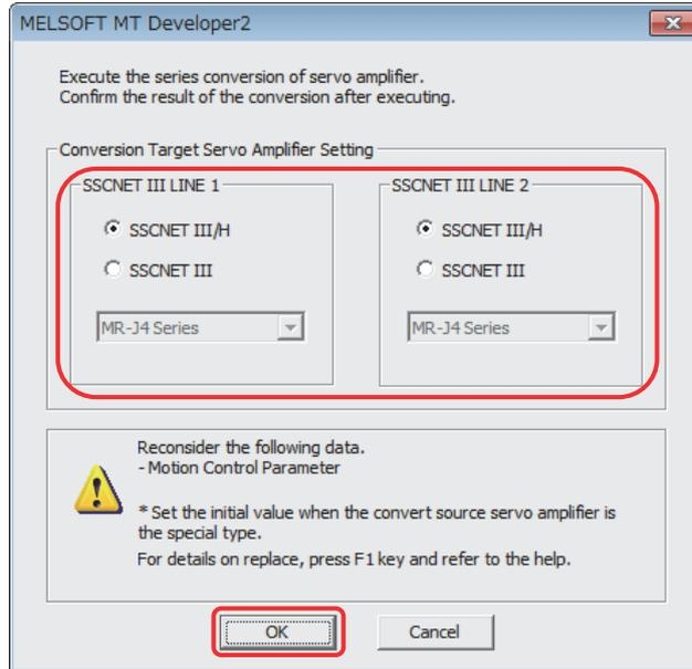
(Note): Refer to “MELSEC iQ-R Motion Controller User’s Manual” for the servo system networks supported by the replaced servo amplifiers and SSCNETIII compatible devices (SSCNETIII or SSCNETIII/H).
