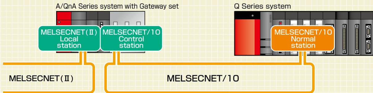
[Example] Step-by-step system replacement to have a system entirely made up with the Q Series
