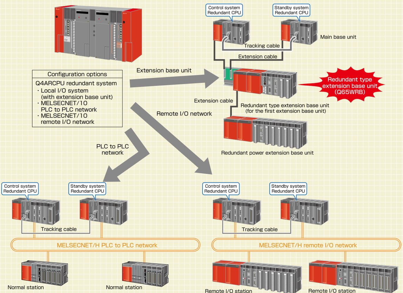
■ Network modules of MELSECNET/H PLC to PLC network and remote I/O network can be installed to the Q Series redundant CPU main base. (They can be used together.)
