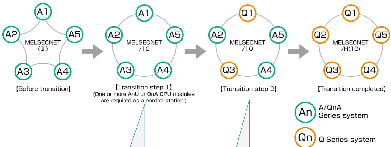
Replace MELSECNET(II) data link modules at all stations with MELSECNET/10 network modules, and then switch the network system over to MELSECNET/10.
