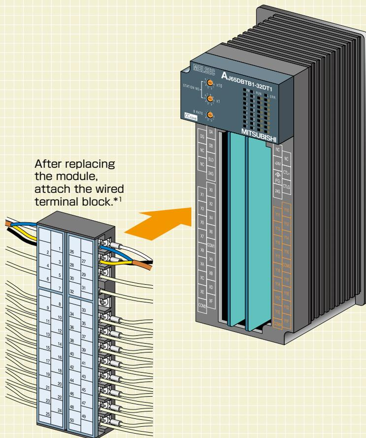
\*1: The communication cables and power cables need to be rewired.
