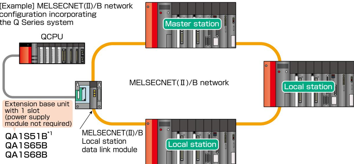
\*1: QA1S51B, which does not have an extension cable connector(OUT), cannot be connected with any other extension unit. QA6□B, or QA6ADP with A5□B/A6□B cannot be used in combination.
