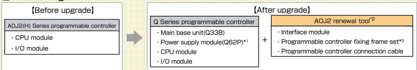
\*1: The interface modules except for some models require 24 V DC power supply. If the Q62P is not used, provide a separate external power supply.
