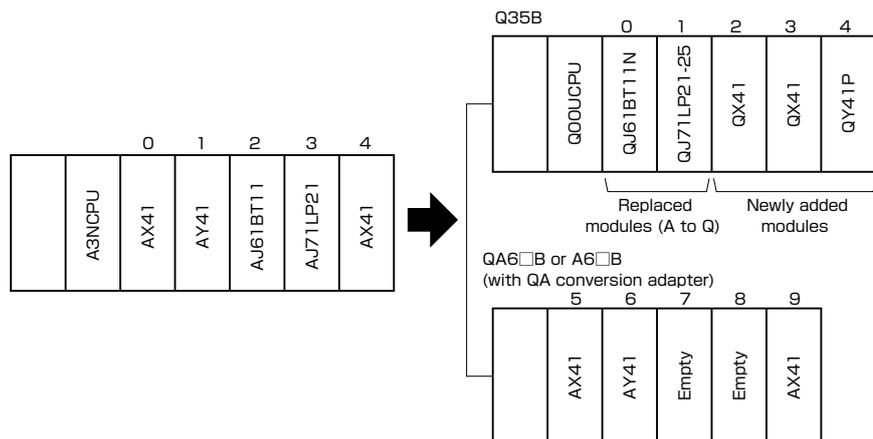
Replace the incompatible A/QnA modules with the Q Series modules.
