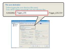
• A folder with the name specified above is created on the CompactFlash card.
