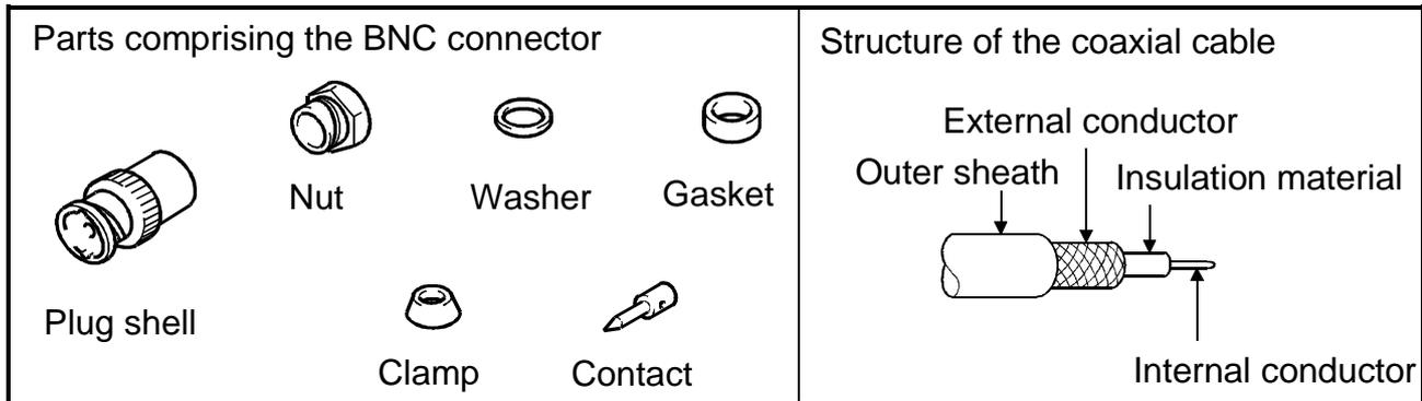
(2) How to connect the BNC connector and the coaxial cable
