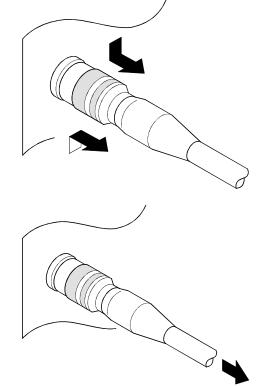
1. Release the lock by pulling the lock release mechanism section of the plug in the direction of the arrows.
