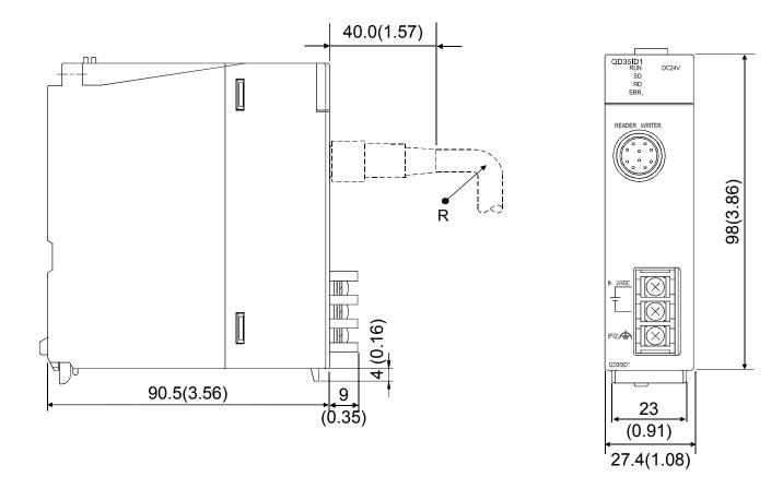
R (Bending radius near connector) : 40mm(1.57 inch)
