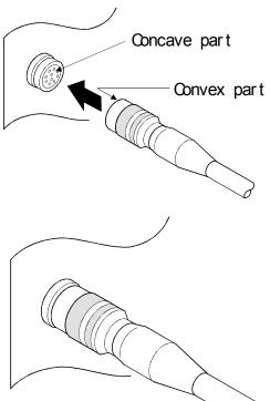
1. Insert the convex part of the plug into the concave part of the jack.
