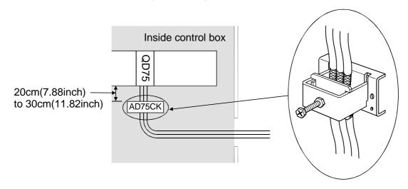
Using the AD75CK, you can tie four cables of about 7mm outside diameter together for grounding.
