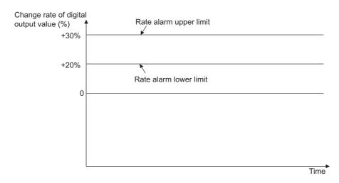
Ex. 2: To monitor a drop rate of a digital output value is within the specified range
