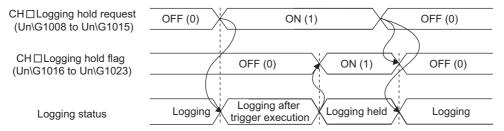
• When OFF (0) is set to CH□ Logging hold request (Un\G1008 to Un\G1015) before ON (1) is stored in CH□ Logging hold flag (Un\G1016 to Un\G1023), the logging does not stop.
