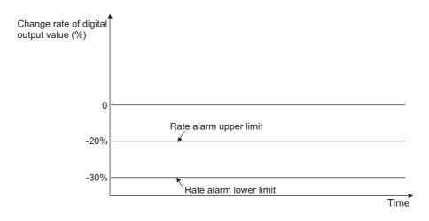
Ex. 3: To monitor a change rate of a digital output value is within the specified range
