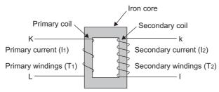
Primary and secondary coils winded an iron core are isolated electrically. When a primary current (I1) is applied to the iron core, a secondary current (I2) can be extracted depending on the turn ratio (current transformation ratio).
