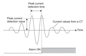
• The number of peak current detection is recorded in a non-volatile memory. Therefore the number of peak current detection is not cleared after turning off the power supply or resetting the CPU module.
