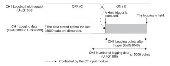
Ex. When CH□ Level trigger condition setting (Un\G1056 to Un\G1063) is set to a value other than Disable (0) and CH1 Digital output value (Un\G11) is logged
