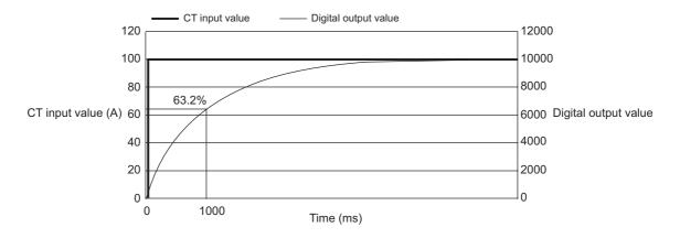
Ex. 2: When CT input values form a ringing waveform, change of digital output values in the following conditions
