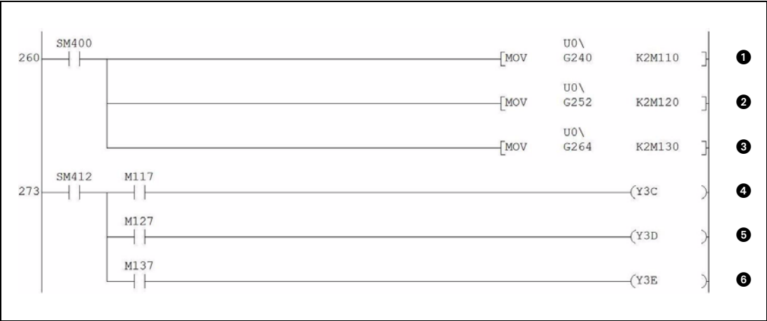
Fig. 5-14: HART field device status check and error processing
