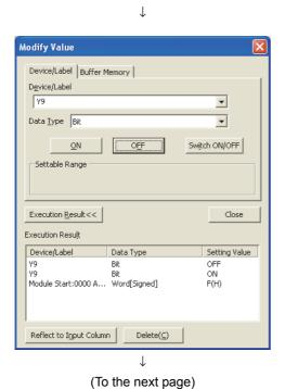
Open the "Device/Buffer Memory Batch Monitor" window.
