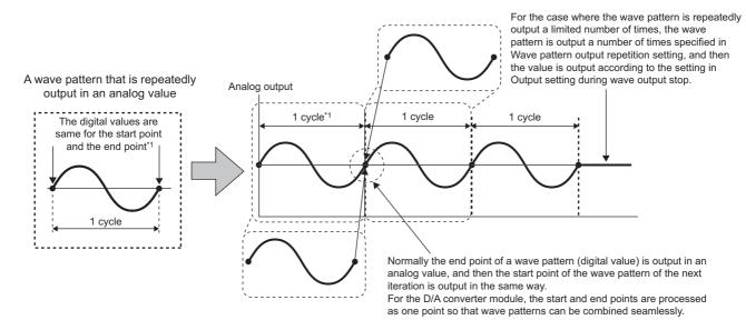
\*1 The output cycle of a wave pattern is calculated by the following formula.
