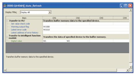
6. Write the set parameters to the remote I/O module and reset the remote I/O module.
