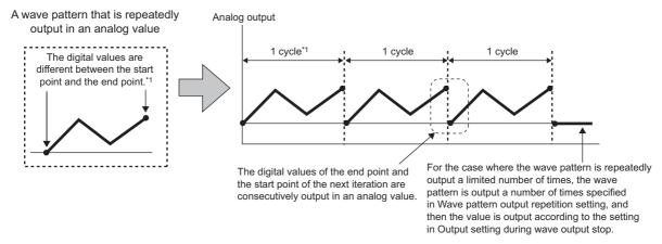
\*1 The output cycle of a wave pattern is calculated by the following formula.
