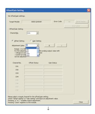
5. The adjustment amount of the offset value or gain value can be selected from "1", "100", "500", "1000", "2000", and "3000" or it can be set by inputting any value (1 to 3000).
