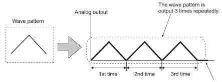
After the wave pattern was output 3 times, wave output stops and an analog value is output according to the setting in CH $\square$  Output setting during wave output stop (Un\G1008 to Un\G1011).
