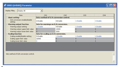
5. Display the auto refresh setting window for the Q64DAH and configure the setting as follows.
