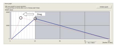
The end point position also can be adjusted by changing the value of "End point" and "Digital value" in "Wave details setting".
