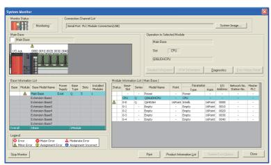
1. Select the D/A converter module in "Main Base" and click the Detailed Information button.
