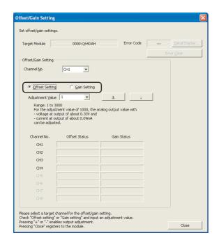
Use the radio button to specify whether the offset setting or gain setting.
