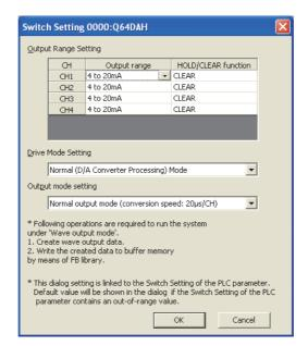
4. Display the initial setting window for the Q64DAH and configure the setting as follows.
