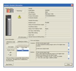
2. "Module's Detailed Information" of the D/A converter module is displayed.
