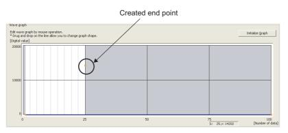
To delete the end point, move the mouse pointer to the point. Then select "Delete end point" from the right-click menu. When the mouse pointer is on the end point, the display of the mouse pointer is changed to +.
