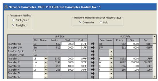
5. Write the set parameters to the CPU module of the master station. Then reset the CPU module or turn off and on the power supply of the programmable controller.
