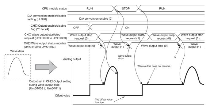
Wave output starts when CH□ Wave output start/stop request (Un\G1000 to Un\G1003) is changed from Wave output stop request (0) to Wave output start request (1).
