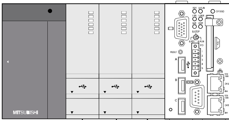
Module No.1 : QCPU (Q mode) Module No.2 through 3 QCPU (Q mode) or motion CPU Constructing a multiple CPU system with up to 3 modules is allowed
