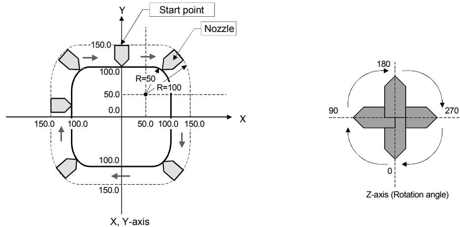
The program to start as the upper figure from start point and which keeps a nozzle at right angles toward the contour of line and that it goes around the contour and which is returned to start point. It is the following program when a helical interpolation function is used.
