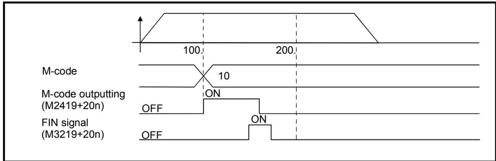
When the FIN signal (M3219+20n) is turned from OFF to ON to OFF during positioning in block 2), the axis performs constant-speed operation without decelerating in the block of M-code.
