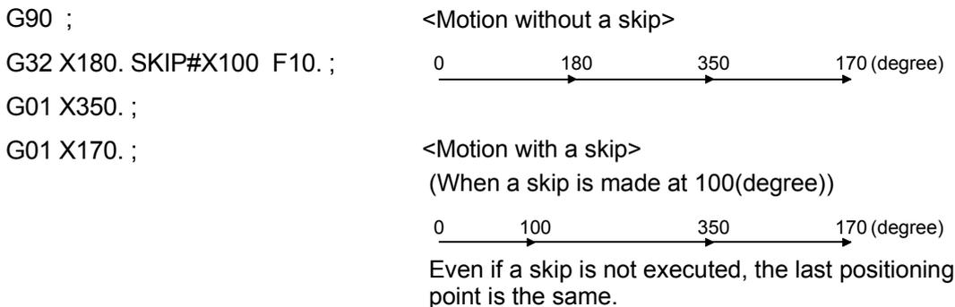
(Note) : The above explanation is valid until a deceleration stop (constant-speed positioning command to point-to-point positioning command, etc.) after skip (G32). After a deceleration stop, operation of the normal [degree] axis is performed. The conditions of deceleration stop after a skip (G32) are shown below. Refer to "6.13.19 G32 Skip" for details.
