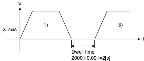
The X-axis is positioned to "100.", stops there for 2[s], and starts positioning operation to "200." again.
