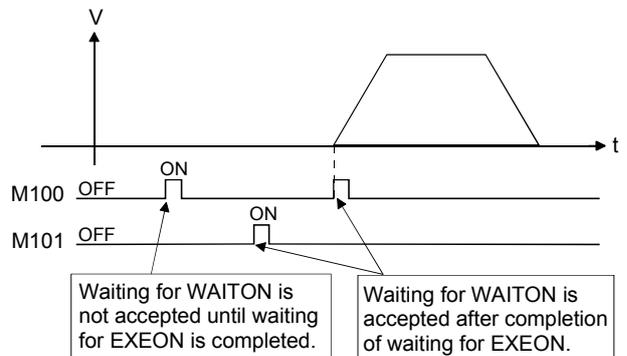
When the EXEON is written in the next block of WAITON (not travel value), priority is given to waiting condition for EXEON regardless of WAITON state, in this case, since an operation is complicated, it recommends not using it combining WAITON and EXEON.
