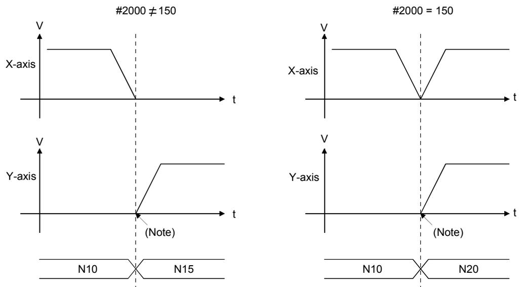
(Note) : When M100 is executed, constant-speed positioning does not continue from N10 to N15 or from N10 to N20 and a deceleration stop is made once after execution of N10.
