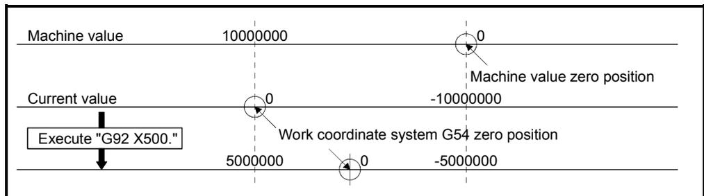
The 0 position of the current value is re-set to 500. , which results in the current value of 5000000.
