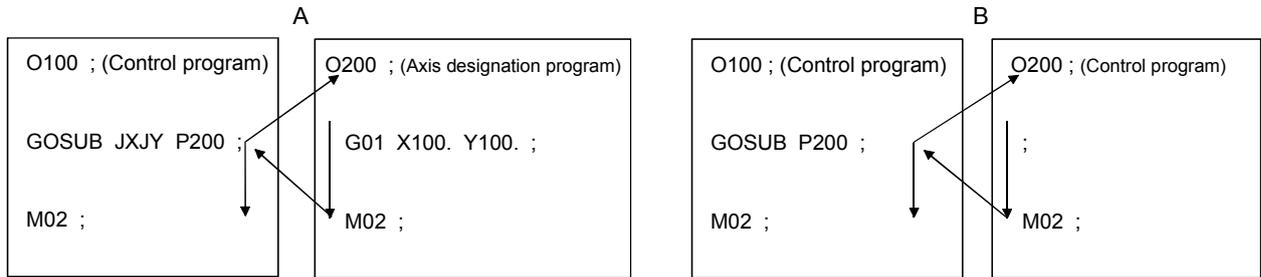
(a) When the started program is a control program, if the main program (O0100) is cleared, the both of the main program (O0100) and subprogram (O0200) end. (Figure B)
