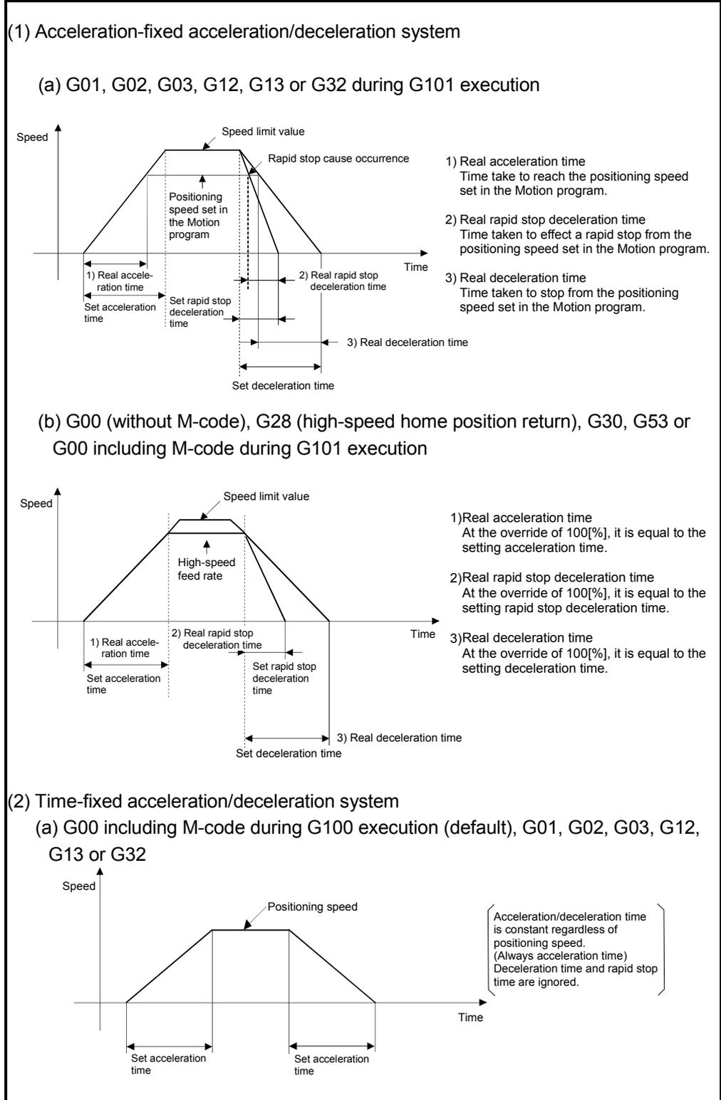
Fig. 5.4 Relationships between the speed limit value, acceleration time, deceleration time and rapid stop deceleration time
