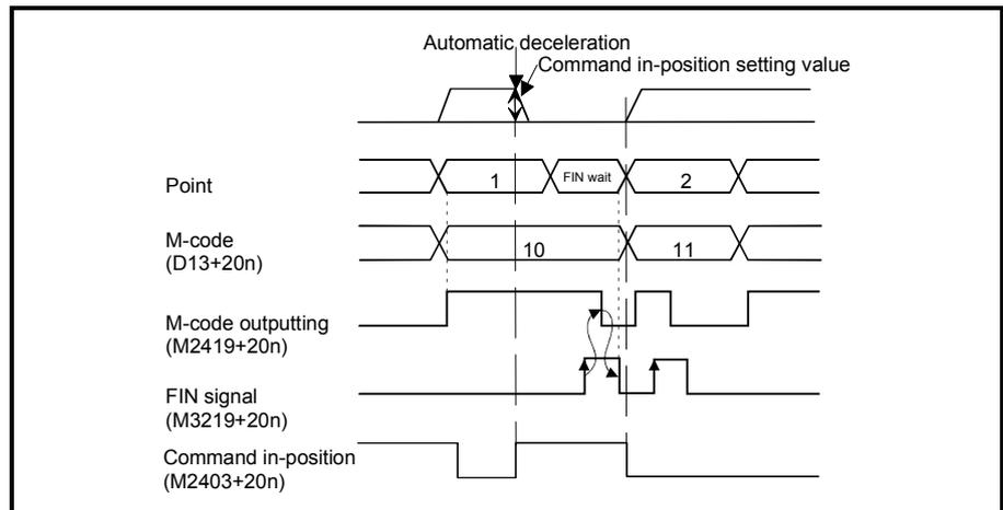
(b) When the axis transits to the next point without automatic deceleration by positioning to the executing point during FIN signal wait.
