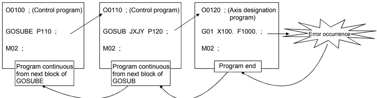
If an error which program ends will occur in the program No.120, program "O0100" and "O0110" execute continuously.
