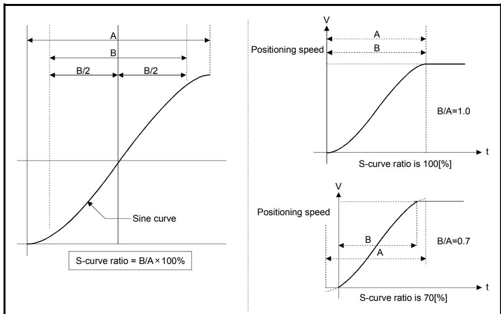
(Note) : When the G00, G01, G02, G03, G12, G13 or G32 including M-code is used, S-curve ratio is ignored and control is executed as always 0[%].
