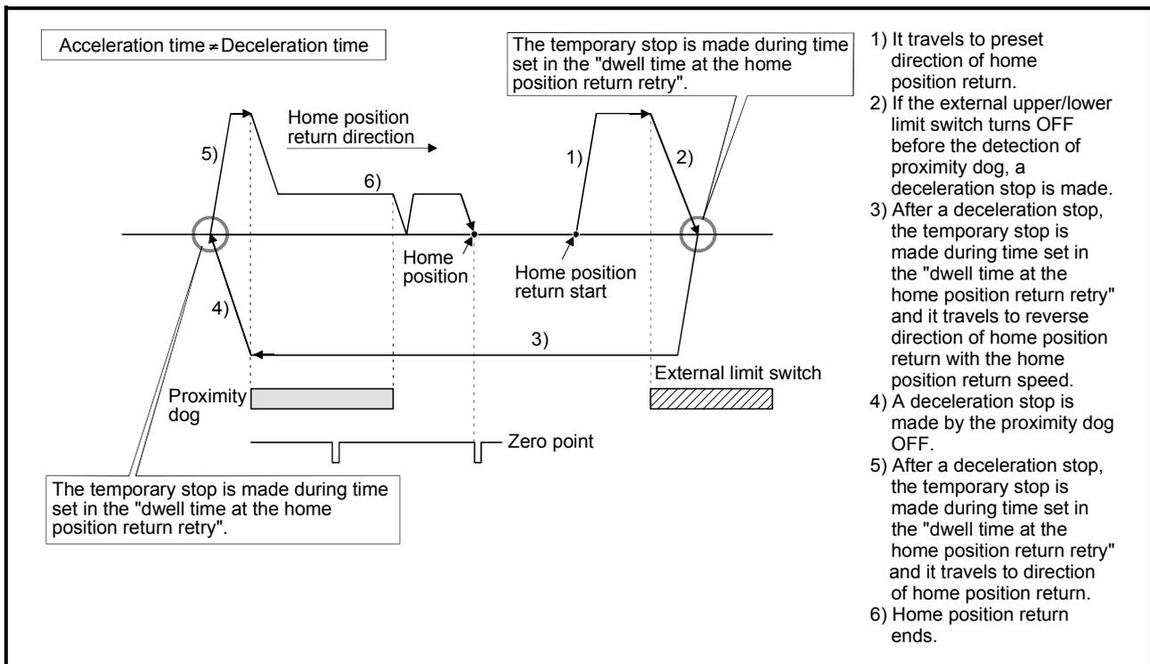
Fig. 7.2 Operation for home position return retry function
