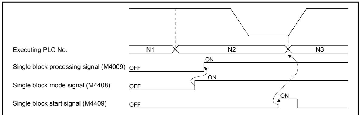
A macro instruction block, e.g. arithmetic operation, is pre-read during execution of the move instruction for PTP (e.g. G00) or CP (e.g. G01). Therefore, if the single block function is executed while the macro instructions are pre-read during motion, the executing block number and executing PLC No. displayed are those in the pre-read area.
