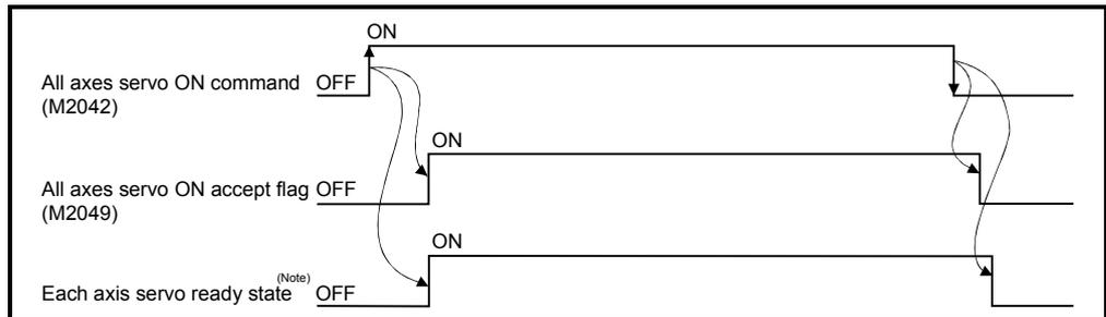
(Note): Refer to "4.1.1 Axis statuses "Servo ready signal"" for details.
