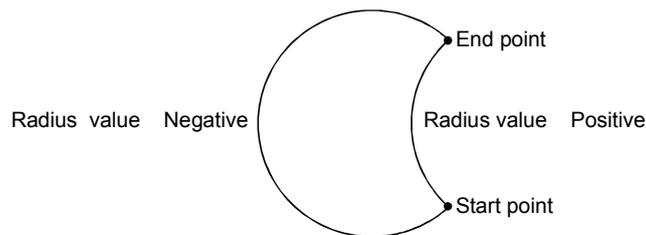
An error will occur if "the distance between start and end points" -  $\text{radius} \times 2 >$  "circular arc error".
