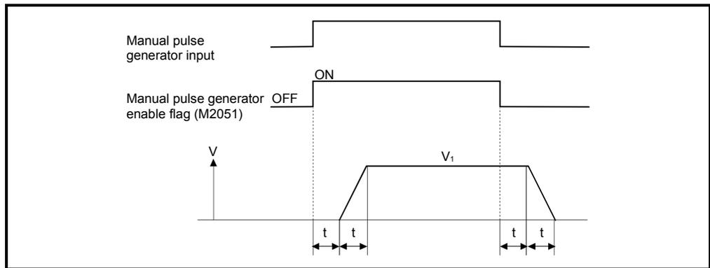
$$\text{Output speed (V1) [PLS/s]} = (\text{Number of input pulses/s}) \times (\text{Manual pulse generator 1-pulse input magnification setting})$$
