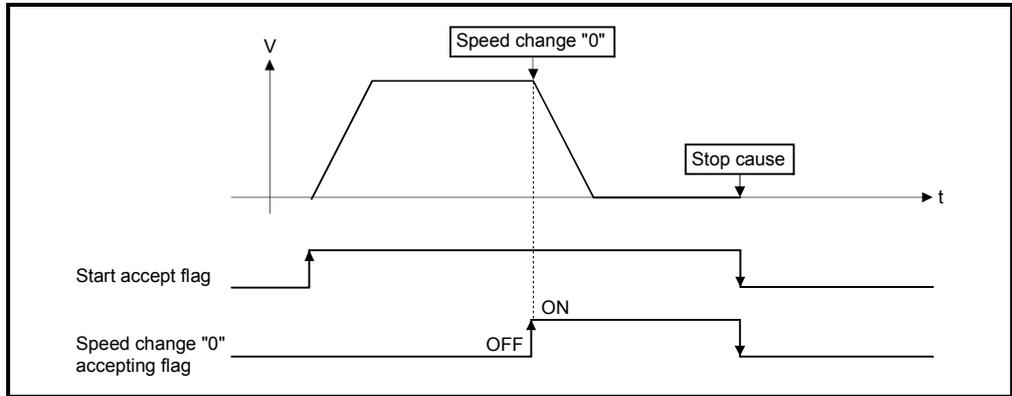
(c) The speed change "0" accepting flag does not turn on if a speed change "0" occurs after an automatic deceleration start.
