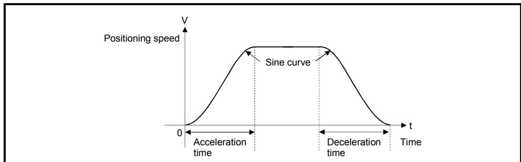
As shown below, the S-curve ratio setting serves to select the part of the sine curve to be used as the acceleration/deceleration curve.
