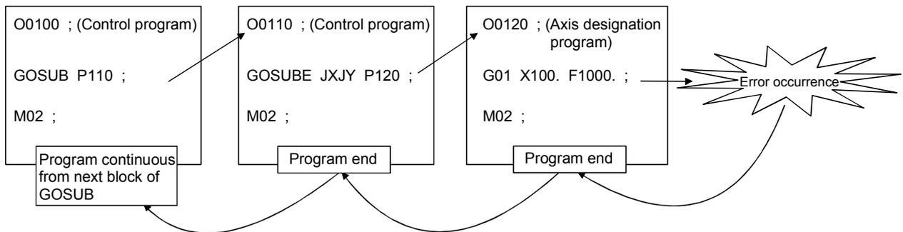
If an error which program ends will occur in the program No.120, program "O0110" ends but program "O0100" executes continuously.
