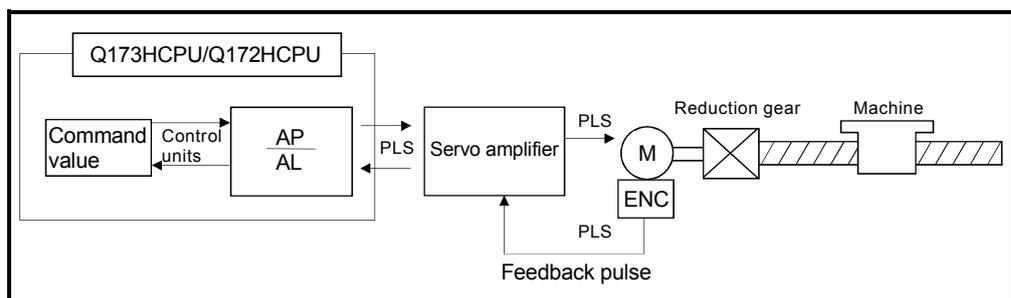
Fig. 5.1 Control content of the Motion CPU
