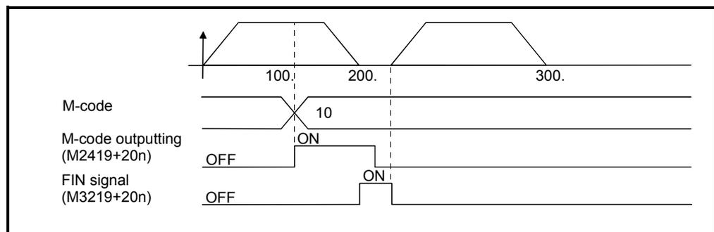
When the FIN signal (M3219+20n) is not turned from OFF to ON to OFF during positioning in block 2), a decelerates stop is made once in the block of M-code.
