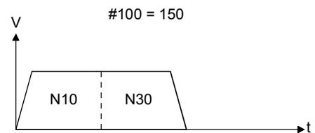
The continuous operation is not executed and a stop once in the preread disable mode as for the G01 continuous block.
