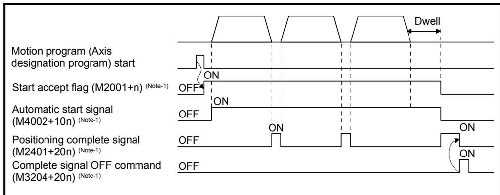
Fig.4.3 ON/OFF timing of the positioning complete signal
