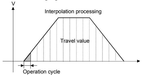
[Command speed 50m/min, Operation cycle 3.5ms]
