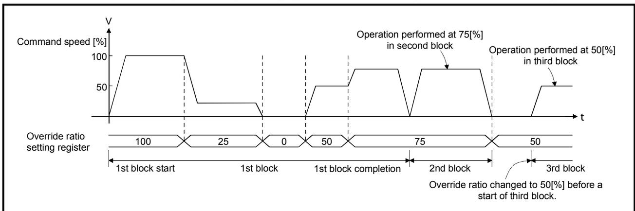
Fig. 7.22 Speed change timing for override ratio setting
