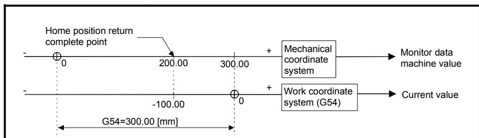
On completion of a home position return, the machine value is equal to 200.00[mm] and the current value is equal to -100.00[mm].
