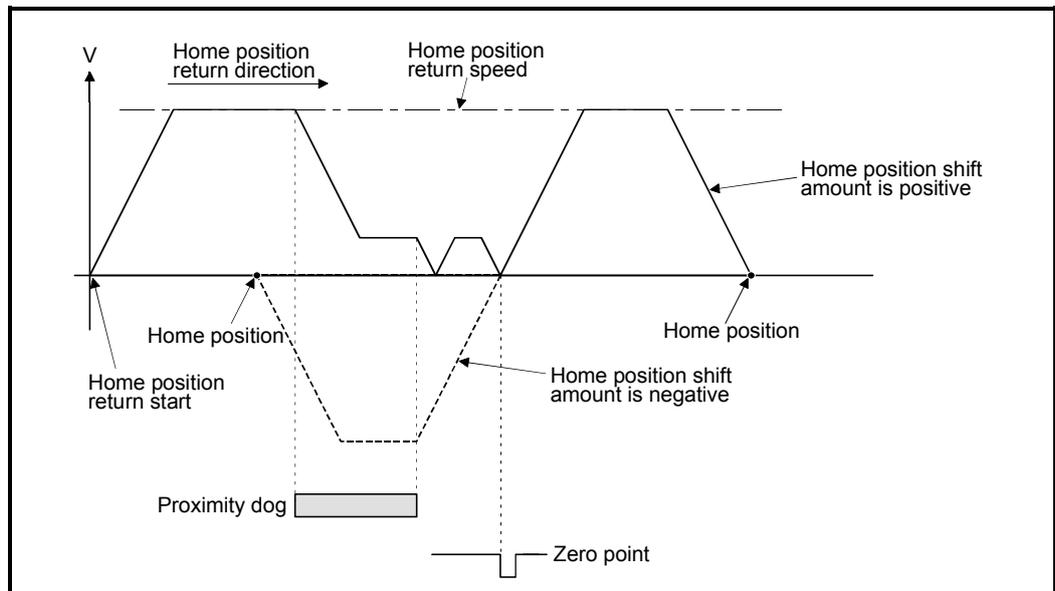
Fig. 7.19 Operation for home position shift with the home position return speed
