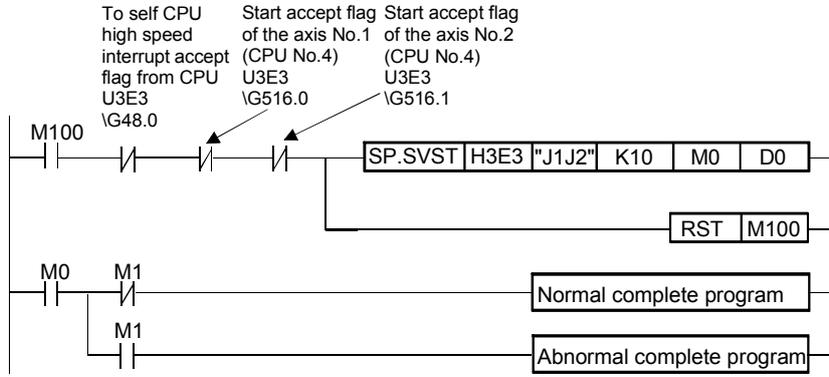
(2) Program which requests to start the Motion program (Axis designation program) No.20, sequence No. 100 and parameter block No.30 toward axis No.1 and No.2 of the Motion CPU No.4 by indirect setting from the PLC CPU No.1.
