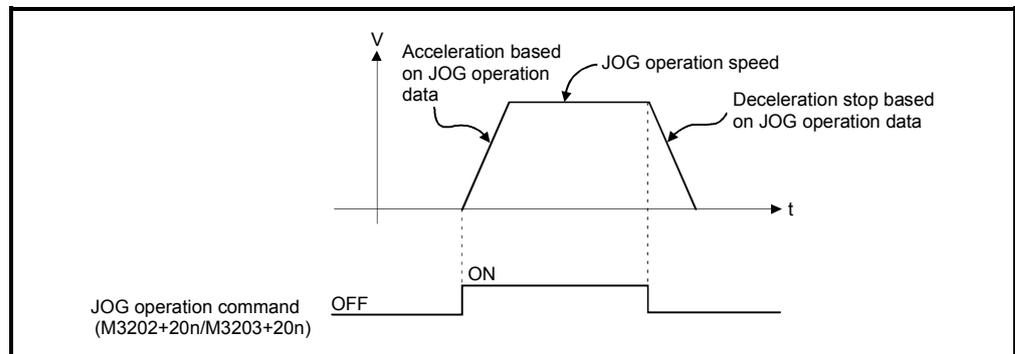
JOG operation for axis for which JOG operation command is turning on is executed.
