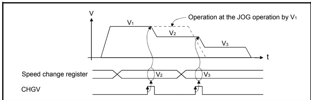
Fig. 7.21 Operation timing for speed change
