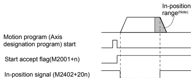
(Note) : If in-position range is longer than the deceleration distance, in-position signal turns on after deceleration start.
