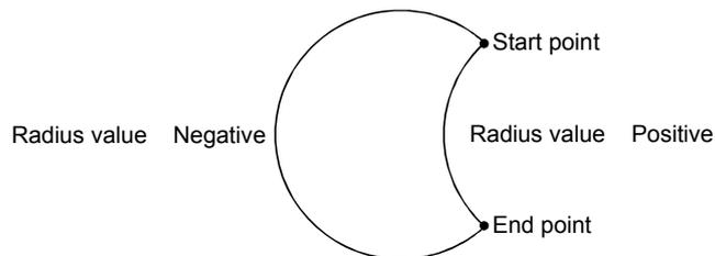
An error will occur if "the distance between start and end points" - radius  $\times$  2 > "circular arc error".
