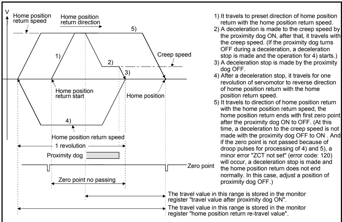
Fig. 7.5 Home position return operation by the proximity dog type 2 (zero point no passing)
