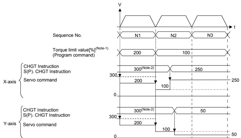
(Note-1) : Indicates the torque limit value change by a program or CHGT/S(P).CHGT instruction, and the resultant command to servo amplifier. Unit is [%].
