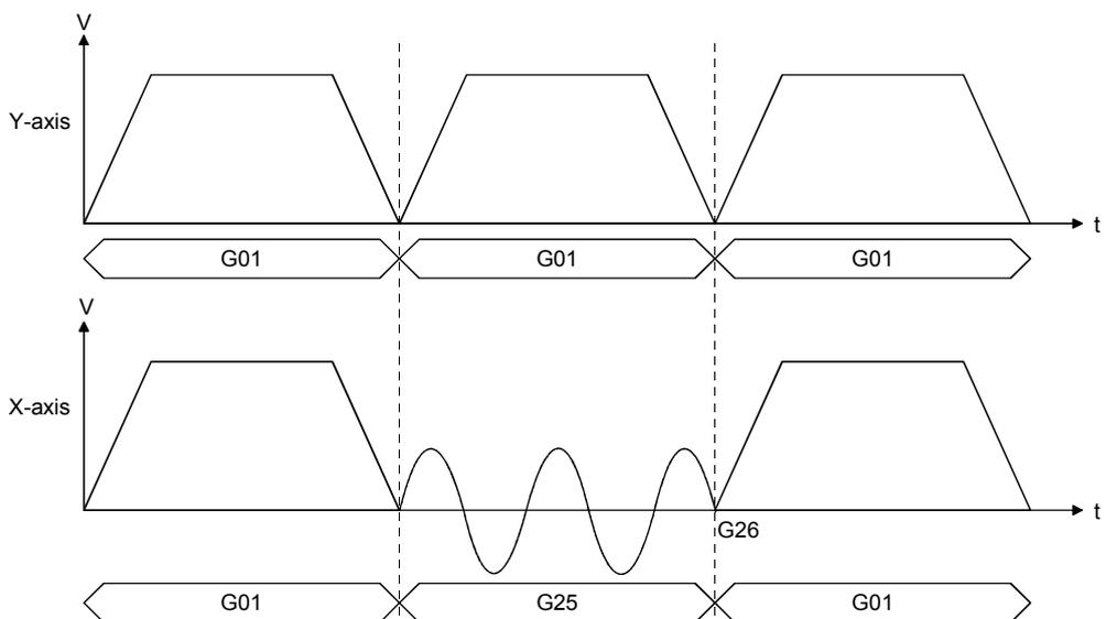
If the start command of the X-axis (high-speed oscillation start axis) is described in the N03 block, a minor error (error code : 581) is displayed when this block is executed, and this program is suspended.
