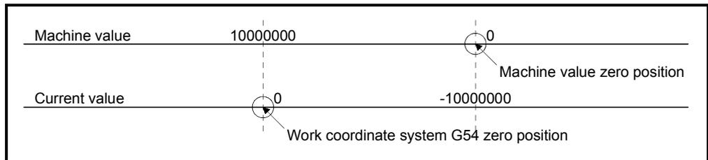
At the 10000000 position of the machine value, the current value is "0".
