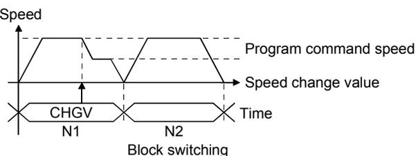
(Note-7): F (speed) command. Note that it is clamped at the speed change value.
