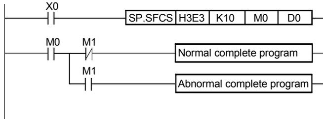
(2) This program starts the Motion program (Control program) No.30 and sequence No.200 of the Motion CPU No.4 by indirect setting.
