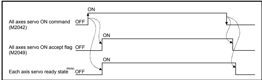
(Note): Refer to "4.1.1 Axis statuses "Servo ready signal"" for details.
