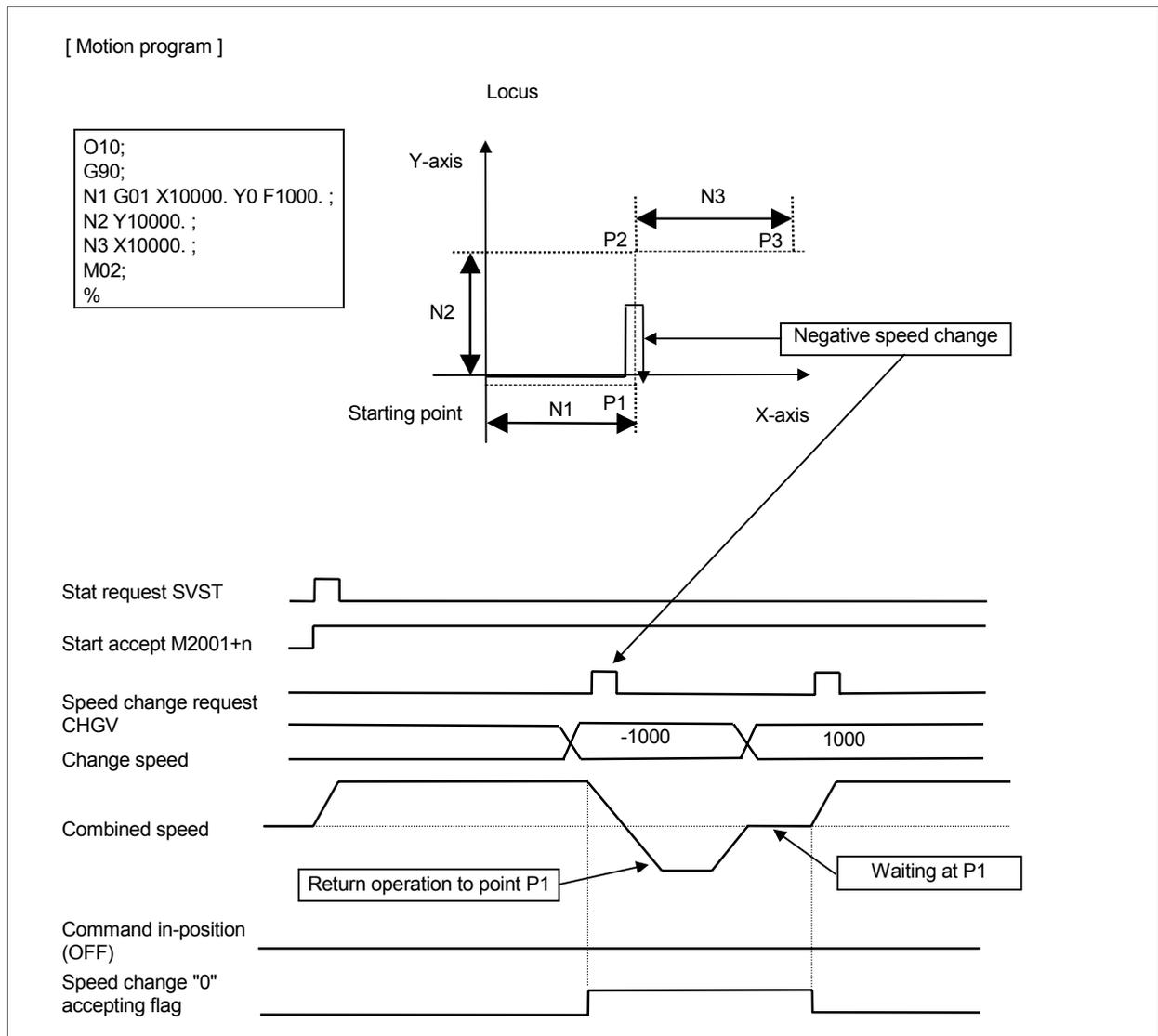
When a speed change is made to negative speed during positioning to P2 in the N2 block as shown above, the axis returns to P1 along the track specified in the program and stands by at P1.
