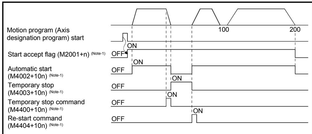
Fig.4.4 ON/OFF timing of the temporary stop signal
