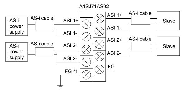
\*1: When the noise environment is bat, the terminal FG is grounded.
