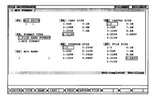
When card size is selected, input standby status is established by pressing the [F4] key.
