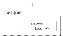
**3** When the [End] key is pressed, an alternative window is shown. With "YES" selection, "Executing [xxx] Sector" is shown and backup is executed.
