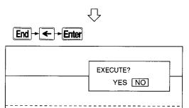
**3** When the [End] key is pressed, an alternative window is shown. With "YES" selection, "Executing" is shown in the message area, and memory card formatting is executed.
