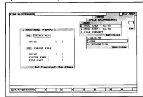
Case of back-up of BASIC data for execution in the memory card in DRIVE "0" to HD with SYSTEM NAME "ABC" and FILE NAME "XYZ" in DRIVE "C".
