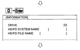
1 Specify the DRIVE containing the memory card, then press the [Enter] key.
