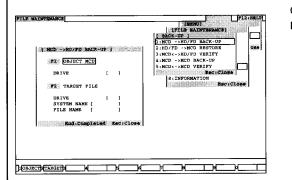
Case of backup of files in the memory card in DRIVE "1" to FD in DRIVE "A" with SYSTEM NAME "ABC" and FILE NAME "XYZ."
