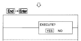
**3** When the [End] key is pressed, an alternative window is shown. With "YES" selection, in the case of HD "Execution [xxx] Sector" is shown in the message area, and in the case of floppy disk, "Executing [xxx] Sector FD No. [n]" is shown, and restoration of the backup file proceeds.
