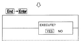
**3** When the [End] key is pressed, an alternative window is shown. With "YES" selection, in the case of HD "Verification [xxx] Sector" is shown in the message area, and in the case of FD, "Verification [xxx] Sector FD No. [n]" is shown, and verification of the backup file proceeds.
