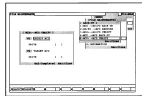
Case of verification of all data in the memory card in DRIVE "0" with the memory card in DRIVE "1".
