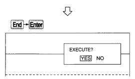
**3** When the [End] key is pressed, an alternative window is shown. With "YES" selection, the "Verify Source Read [xxx] Sector" or the "Verify Destination Read [xxx] Sector" is shown in the message area, and file verify is executed.
