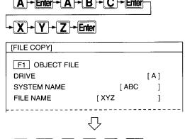
1 Specify the DRIVE, SYSTEM NAME and FILE NAME of the OBJECT FILE and press the [Enter] key.
