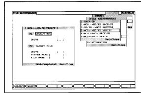
Case of verification of all data in the memory card in DRIVE "1" with the file in DRIVE "C" having SYSTEM NAME "ABC" and FILE NAME "XYZ".
