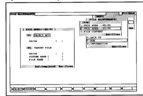
Case of verification of BASIC data for execution in memory card in DRIVE "0" against BACK-UP file with SYSTEM NAME "ABC" and FILE NAME "XYZ" in DRIVE "C".
