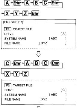
1 Specify the DRIVE, SYSTEM NAME and FILE NAME of the OBJECT FILE and press the [Enter] key.
