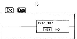
**3** When the [End] key is pressed, an alternative window is shown. With "YES" selection, in the case of HD "Executing [xxx] Sector" is shown in the message area, and in the case of floppy disk, "Executing [xxx] Sector FD No. [n]" is shown, and creation of the backup file proceeds.
