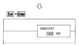
3 When the [End] key is pressed, an alternative window is shown. With "YES" selection, the "Read [xxx] Sector" or the "Write [xxx] Sector" is shown in the message area, and file copy is executed. When the display changes to "Completed," file copy is completed. With "NO" selection, specification can be made again from the copy source drive.
