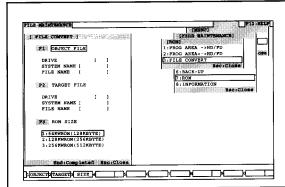
Case of file conversion from backup file with "128KWROM (256KBYTE) ROM size, SYSTEM NAME "ABC" and FILE NAME "XYZ" in DRIVE "A" to file with "128KWROM (256KBYTE) ROM SIZE, SYSTEM NAME "ABC" and FILE NAME "XYZ" in DRIVE "C".
