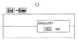
When the [End] key is pressed, an alternative window is shown.
