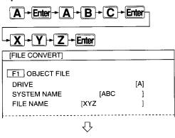
1 Specify the OBJECT DRIVE, SYSTEM NAME and FILE NAME, then press the [Enter] key.
