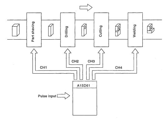
(1) In limit switch output, up to 8 channels can be used.
