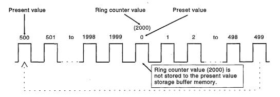
(b) When the preset value of the storage buffer memory (addresses 6 to 7) is set to 2000, the ring counter value of the storage buffer memory (addresses 8 to 9) to 0, and the present value of the storage buffer memory (addresses 0 to 1) to 500 respectively, the ring counter is executed as shown below:
