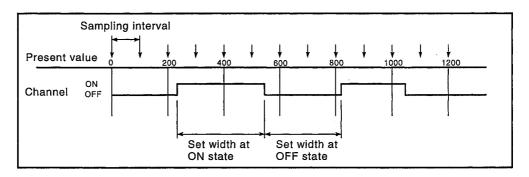
In the A1SD61, the position data is sampled at intervals of 1.0ms and compared them with the set ON/OFF data to output the limit switch signal.
