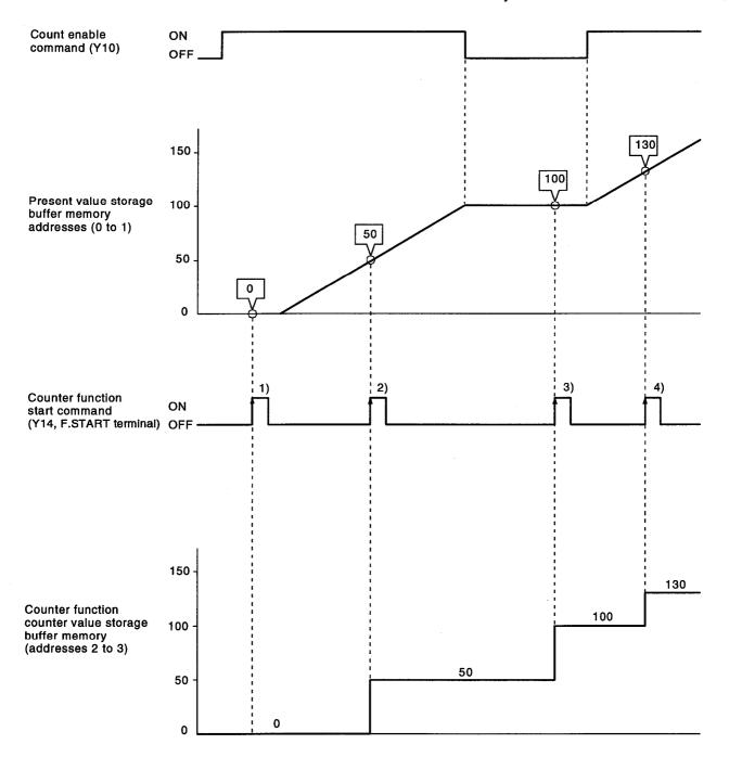
At the rise of the counter function selection start command (Y14, F.START terminal)(corresponding to 1) to 4) in the above diagram), the counter present value is stored to the counter function selection count value buffer memory (addresses 2 to 3).
