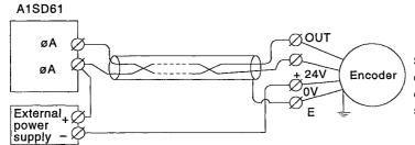
Since currents flow in the twisted pair cable in the same direction, a canceling effect is lost and the module becomes susceptible to electromagnetic induction.
