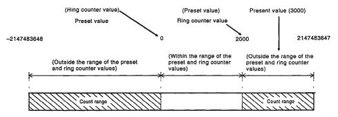
When the preset value storage buffer memory (addresses 6 to 7) is set to 0, the ring counter value storage buffer memory (addresses 8 to 9) to 2000, and the present value storage buffer memory (addresses 0 to 1) to 3000 respectively, the ring counter is executed as shown below:
