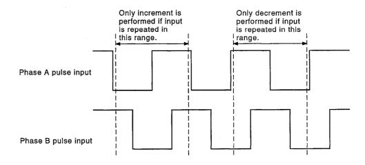
(2) When the use of such increment and decrement as positioning control is required, it is recommended to use multiplication by four.
