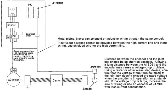
• Ground twisted shielded wire on the encoder side (joint box). (This is a connection example for 24 V send load.)
