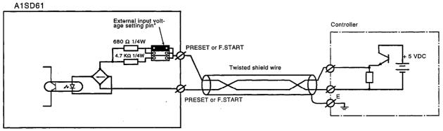
This diagram assumes that the internal circuit is set to PRESET.
