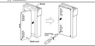
To install the shield cover to the module, install the cover to the terminal side first as shown in the figure, then it will be completed by pushing the cover to the module and tightening the shield fixing screw
