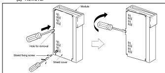
To remove the cover from the module, remove the shield fixing screw first and insert the tip of a flat-tip screwdriver into the removal hole as shown in the figure, then move the screwdriver towards the rear of the module to separate the clip from the removal hole and remove the cover.
