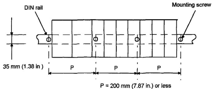
3. Mounting base unit onto DIN rail
