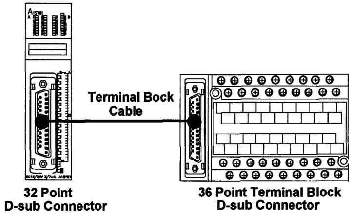
Remote terminal block units for use with connector wiring type input and output modules. Connected to the I/O modules using a terminal block cable. There are many types of terminal block unit with a differing number of terminal points and/or compatible with different I/O modules.
