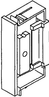
The memory modules allow EEPROMs and EPROMs to be used for program storage, in addition to the RAM memory in the CPU module.
