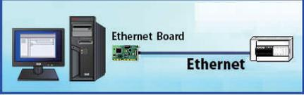
Directly communicate with the CPU module without using a hub.
