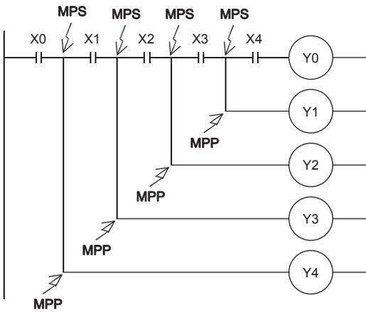
By changing the circuit as follows, the same contents can be programmed easily without MPS instruction.
