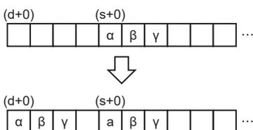
As the result of string conversion, the device ranges do not overlap, and the program terminates normally.
