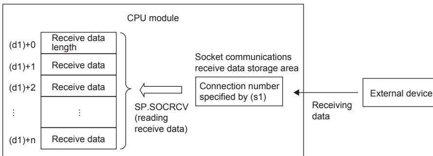
The completion of the SP.SOCRCV instruction can be checked using the completion devices (d2)+0 and (d2)+1.
