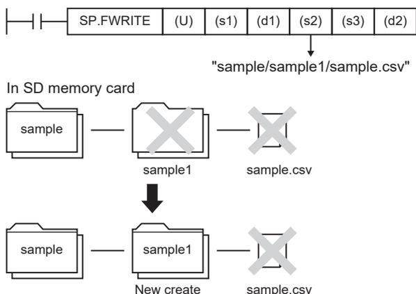
The specified folder path will be created, and the processing will be terminated. When the folder exists, no processing will be performed.
