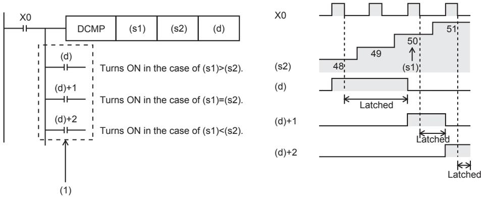
(1): Even if the command input turns OFF and the DCMP instruction is not executed, (d) to (d)+2 latches the status just before the command input turns from ON to OFF.
