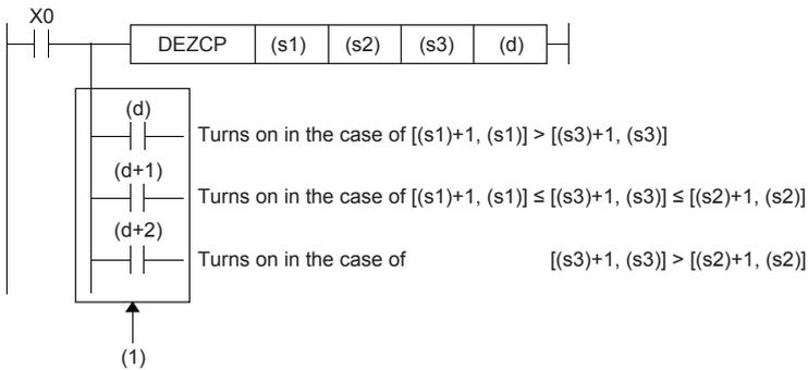
(1): Even if the command input X0 turns off before the DEZCP instruction is fully executed, (d) to (d)+2 hold the status.
