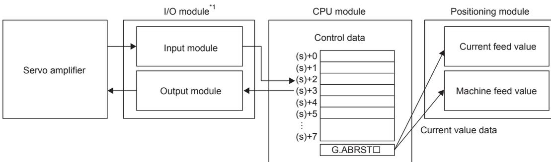
\*1 The CPU module input/output can also be used.
