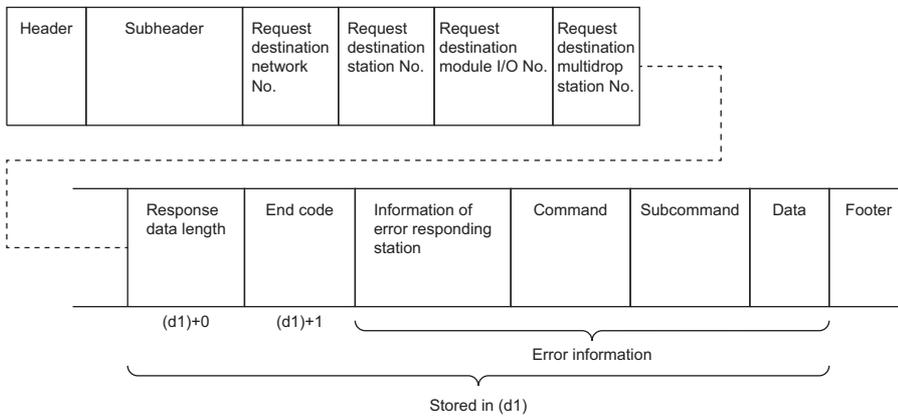
The network number, station number, request destination module I/O number, and multidrop station number are stored to the information of the error responding station.
