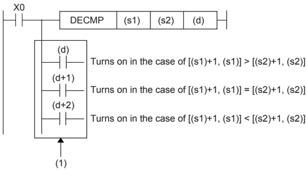
(1): Even if the command input X0 turns off before the DECMP instruction is fully executed, (d) to (d)+2 hold the status.
