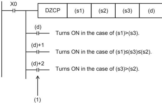
(1): Even if the command input turns OFF and the DZCP instruction is not executed, (d) to (d)+2 latches the status just before the command input turns from ON to OFF.
