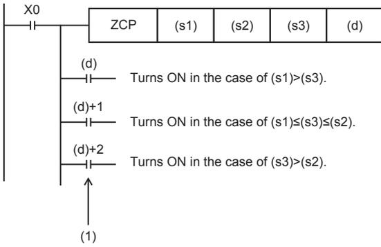
(1): Even if the command input turns OFF and the ZCP instruction is not executed, (d) to (d)+2 latches the status just before the command input turns from ON to OFF.
