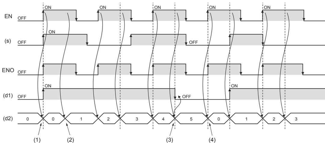
(1): When EN and (s) are on, (d1) turns on. When EN and (s) are on, the time measurement of (d2) starts.
