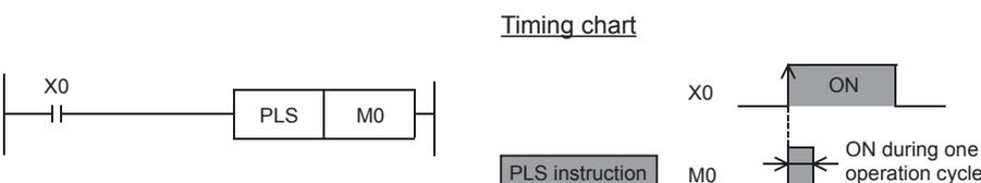
In the figure above, M0 is ON during only one operation cycle when X0 changes from OFF to ON.
