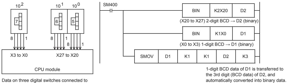
Data on three digital switches connected to non-consecutive input terminals are composed.
