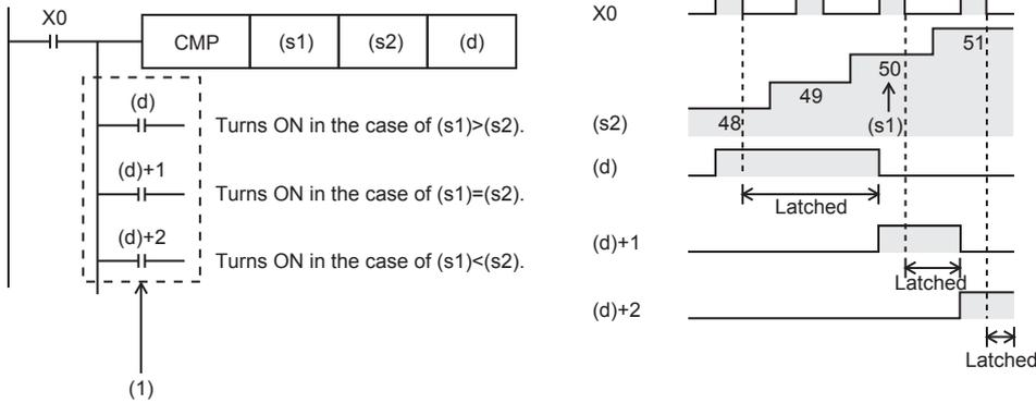
(1): Even if the command input turns OFF and the CMP instruction is not executed, (d) to (d)+2 latches the status just before the command input turns from ON to OFF.
