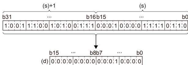
The total of 1 is stored in the binary data. (In the example shown on the left, the total is 16.)
