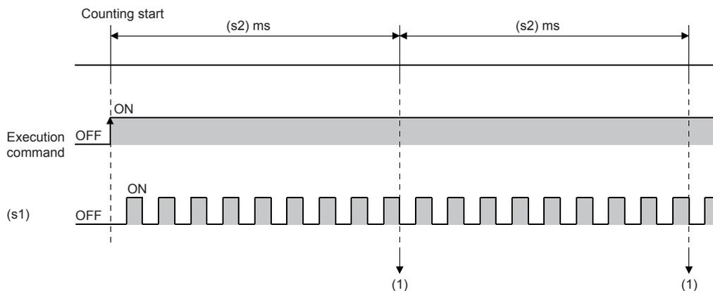
(1): The elapsed time is judged using the 1ms interrupt and the counted result is stored in (d).
