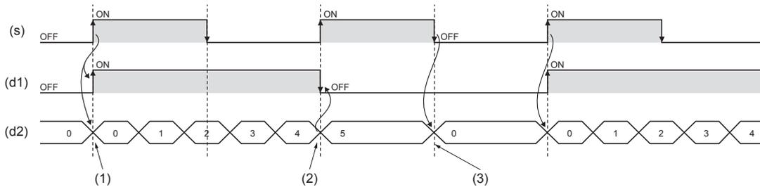
(1): When (s) is on, (d1) turns on. When (s) is on, the time measurement of (d2) starts.
