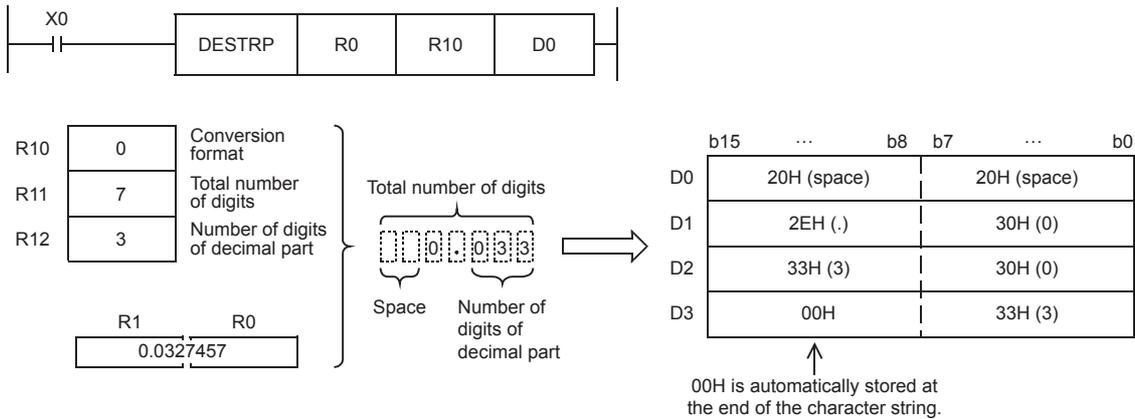
In the program shown below, the contents (single-precision real number data) of R0 and R1 are converted according to the contents specified by R10 to R12, and then stored to D10 and later when X0 turns ON.
