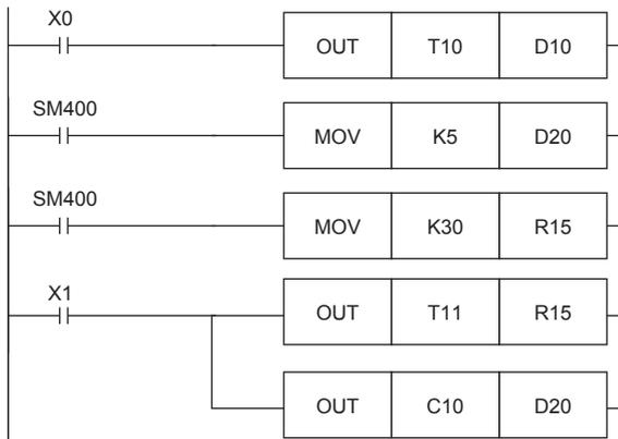
The set value of a timer or counter can be set by a data register (D) or file register (R). At this time, the current value of the data register (D) or file register (R) is regarded as the set value of the timer or counter.
