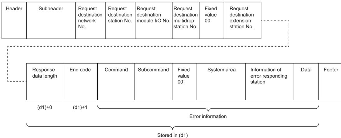
The network number, station number, request destination module I/O number, multidrop station number, 00 (fixed value), and extension station number are stored to the information of the error responding station.
