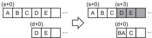
If the overlap of the device ranges is detected in advance, the string to the overlapped point is converted and written to (d). Since the overlap of the device ranges in (s+3) is revealed in advance, the string in (s+0) to (s+2) is converted and written to (d+0) and (d+1). An overlap error (2821H) occurs.
