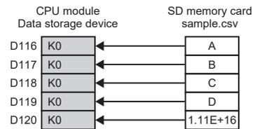
0 is stored in D111 and D114 because -32769 and 65536 are out of the range. 0 is stored in D116 to D120 because all are strings or out of the range.
