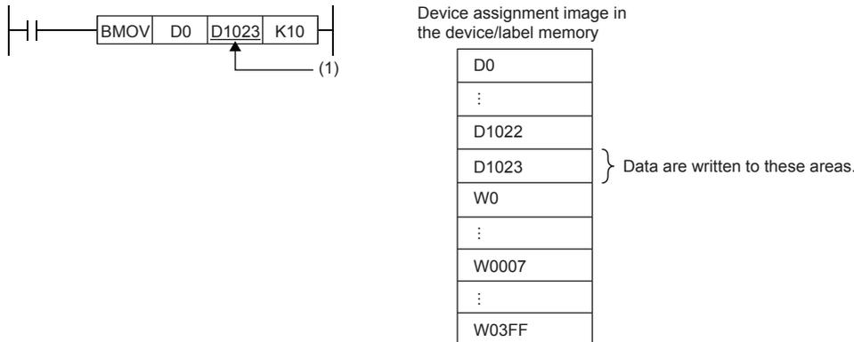
(1) The transfer destination is in the range corresponding to D1023 to D1032. Because D1024 to D1032 do not exist, the data are written only to D1023.
