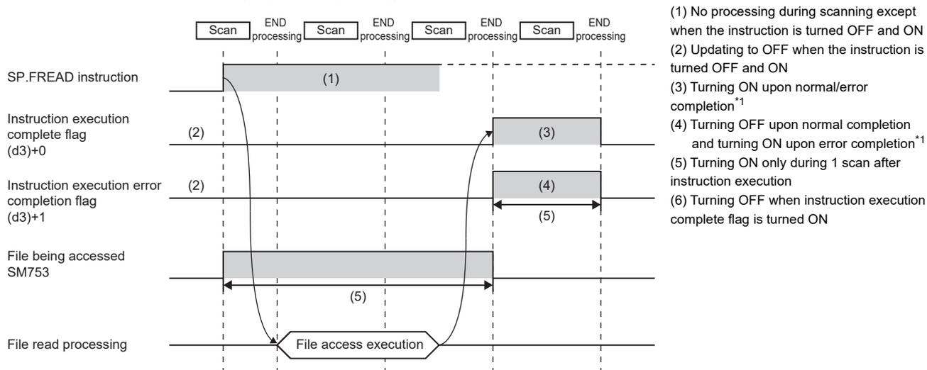
\*1 The complete flag is not turned ON when an error is detected during instruction execution.
