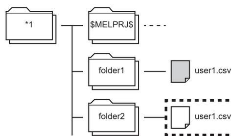
Since the copy destination contains a file with the same name, the file is not copied. The SP.FCOPY instruction is completed normally. When the copy destination does not contain a file with the same name, the file is copied.
