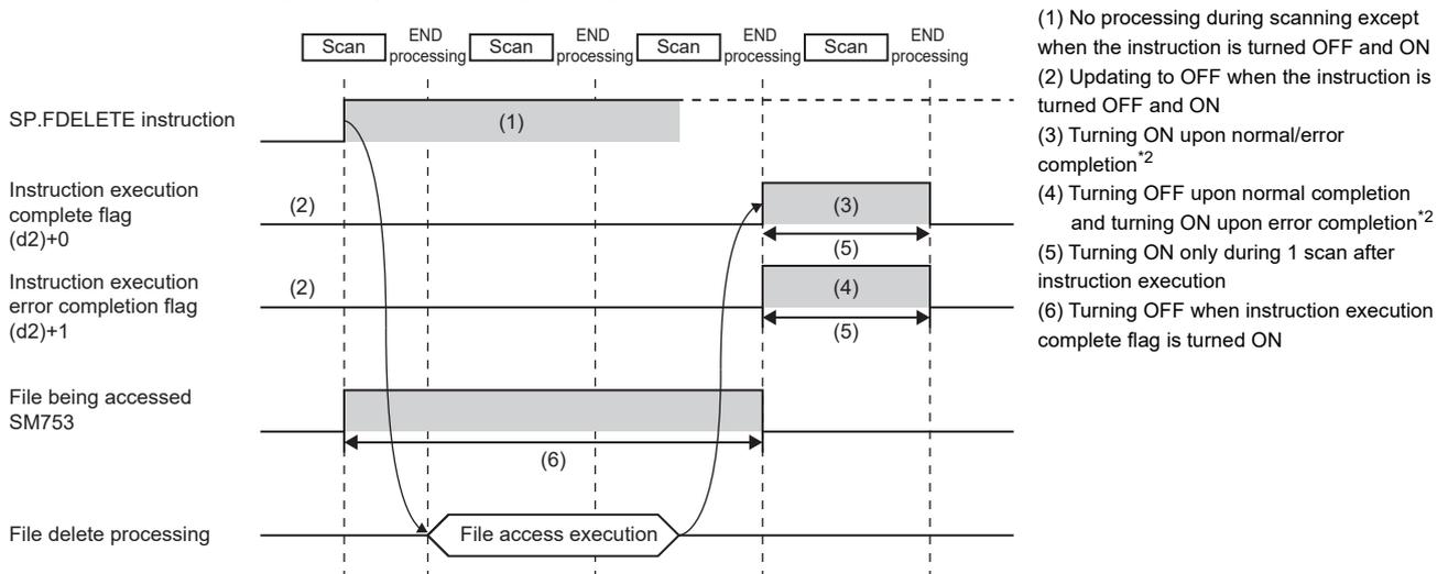
\*2 The complete flag is not turned ON when an error is detected during instruction execution.
