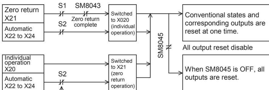
Even if the mode is switched from automatic operation to zero return operation while S2 is ON, state relays (except initial state relays) and outputs are not reset.
