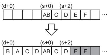
Since the device ranges overlap when the string in (s+2) is converted, the next destination to store is not found. An overlap error (2821H) occurs.
