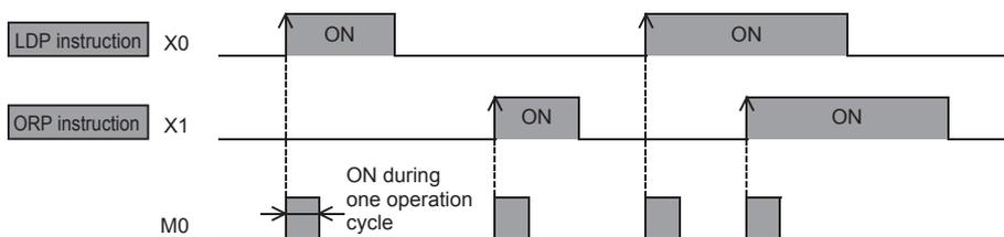
In the example shown above, M0 is ON during only one operation cycle when X0 or X1 turn from OFF to ON.
