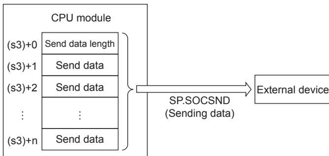
The completion of the SP.SOCSND instruction can be checked using the completion devices (d)+0 and (d)+1.
