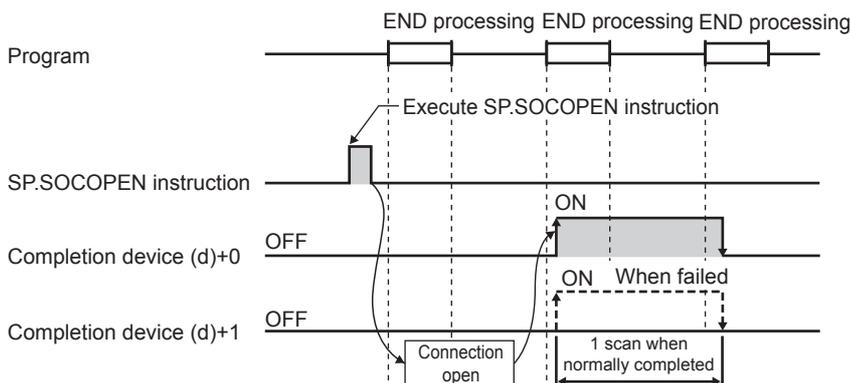
The connection in which no protocol is set with the parameter can be opened and used. In this case, specify 8000H in (s2)+0 and the contents of the open processing in (s2)+2 to (s2)+6.
