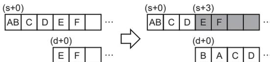
If the overlap of the device ranges is detected in advance, the string to the overlapped point is converted and written to (d).
