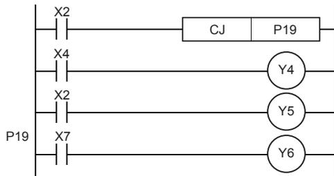
When X2 turns on, the program jumps to the label, P19. Y4 and Y5 remain the same even if X2 and X4 turn on/off during the execution of the CJ instruction.
