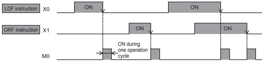
In the example shown above, M0 is ON during only one operation cycle when X0 or X1 turn from ON to OFF.
