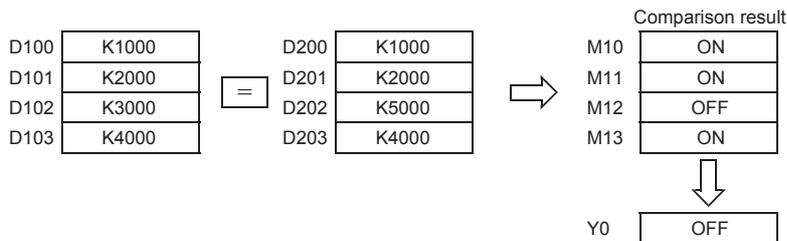
(When all of M10 to M13 are ON, Y0 is set to ON.)
