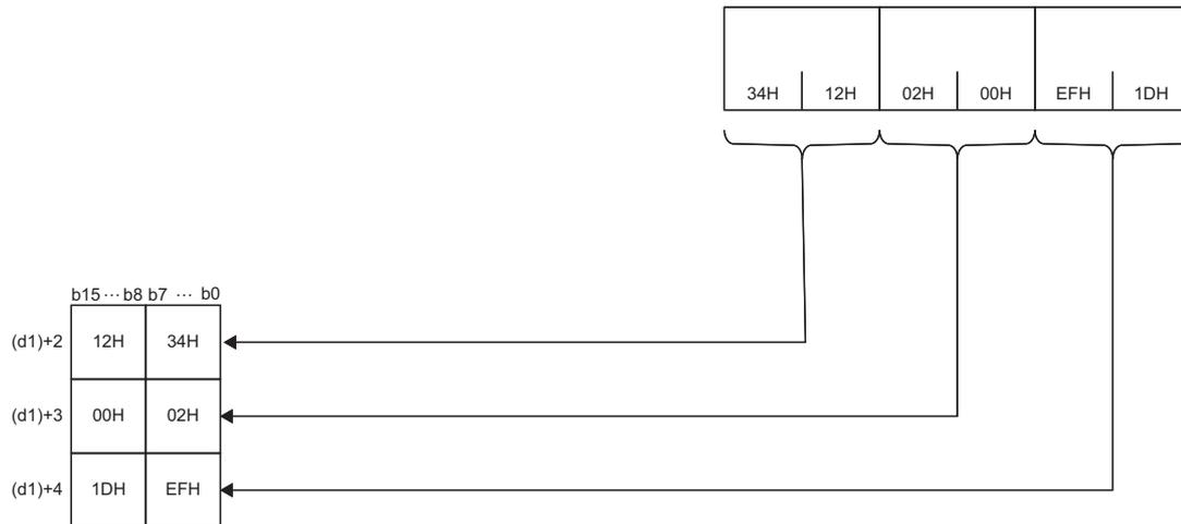
● The following example shows that request data is stored in (s2)+2 and later (station number extension frame).
