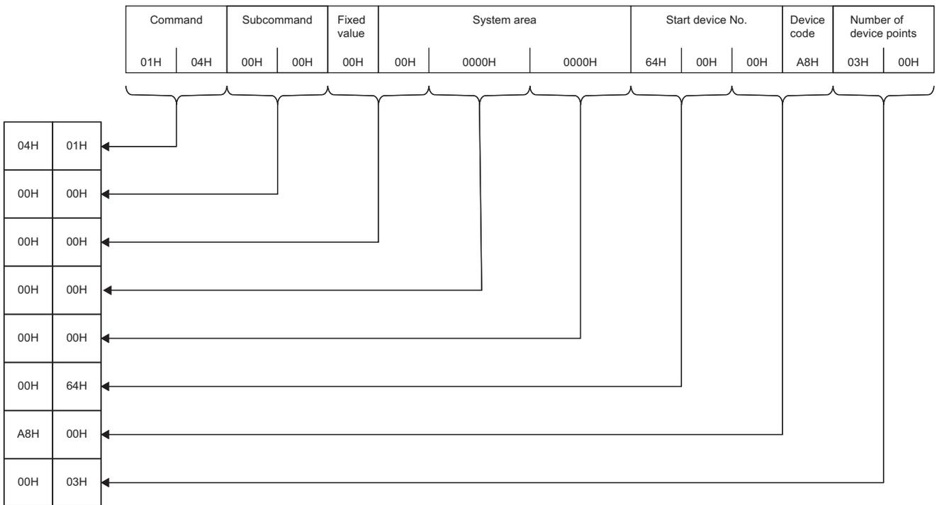
● The following example shows that response data is stored in (d1)+2 and later (station number extension frame).
