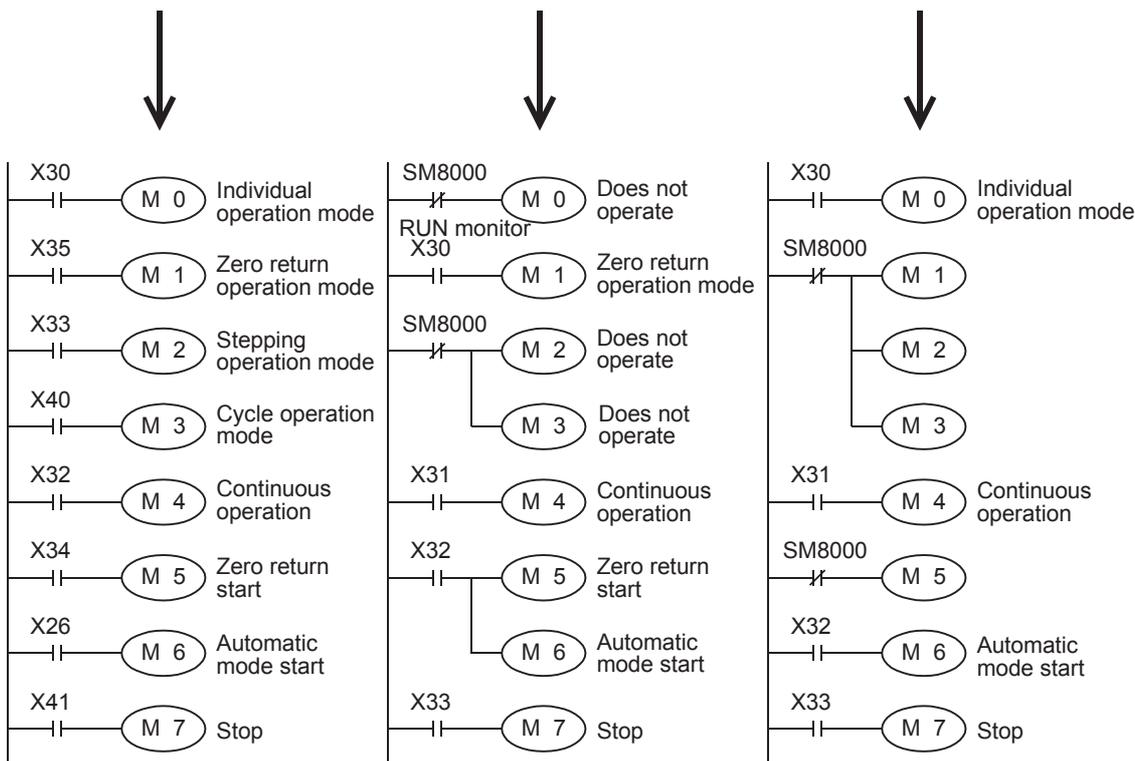
In this example, M0 is used as the head input for mode specification.
