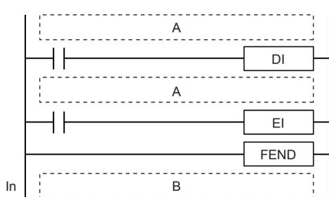
Even though an interrupt occurs between the DI and EI instructions, the execution of the interrupt is held until the processing between the instructions ends.
