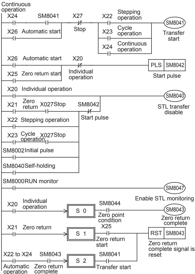
SM8041 is set to ON when the start button is pressed in the automatic mode. Especially in the continuous mode, SM8041 holds its status by itself, and is reset when the stop button is pressed.
