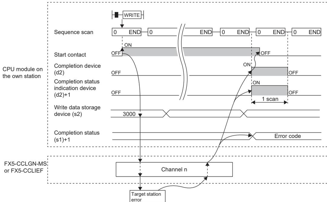
• Write processing is performed only once on the rising edge when the write command turns on.
