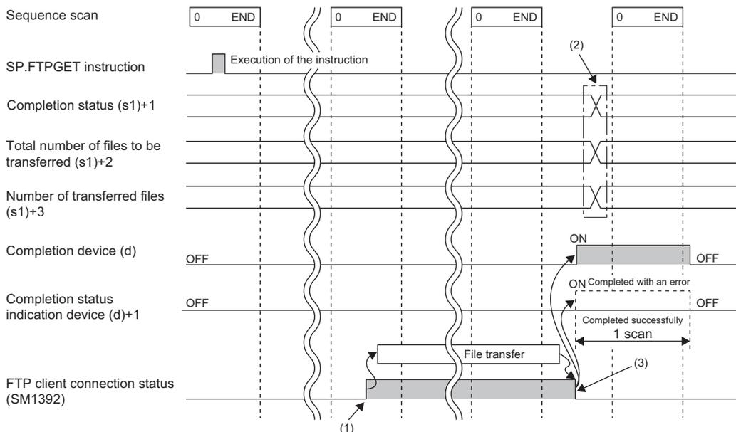
(1) SM1392 turns on during the END processing after the CPU module is connected to the FTP server.
