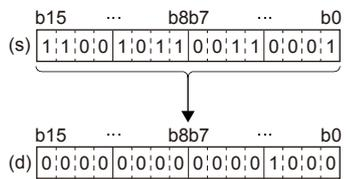
The total of 1 is stored in the binary data. (In the example shown on the left, the total is 8.)
