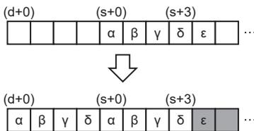
Since the device ranges overlap when the string in (s+3) is converted, the next destination to store is not found. An overlap error (2821H) occurs.
