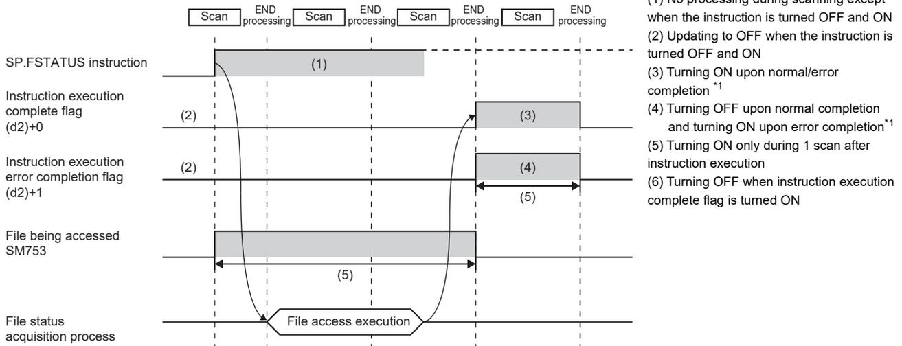
\*1 The complete flag is not turned ON when an error is detected during instruction execution.
