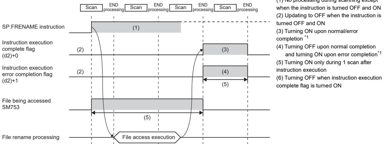
\*1 The complete flag is not turned ON when an error is detected during instruction execution.
