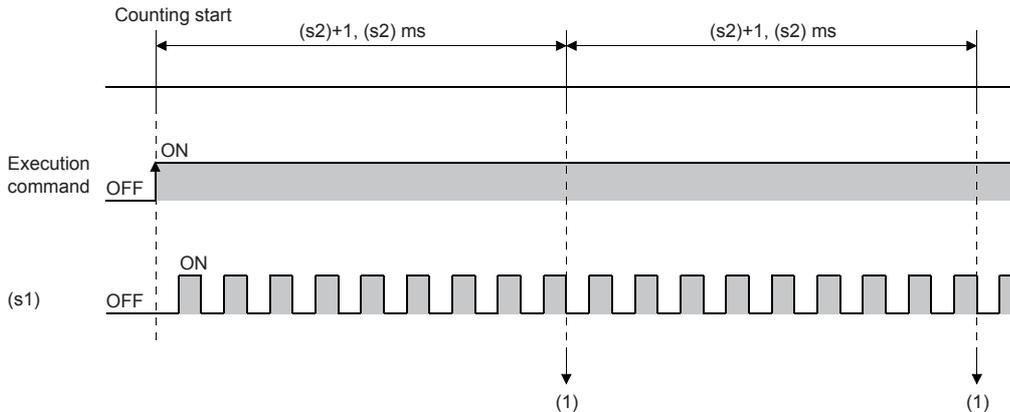
(1): The elapsed time is judged using the 1ms interrupt and the counted result is stored in (d)+1 and (d).
