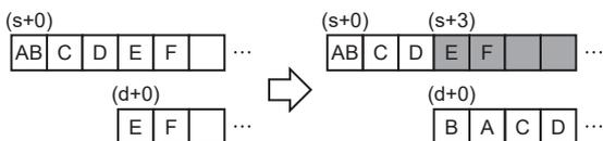
If the overlap of the device ranges is detected in advance, the string to the overlapped point is converted and written to (d). Since the overlap of the device ranges in (s+3) is revealed in advance, the string in (s+0) to (s+2) is converted and written to (d+0) to (d+3). An overlap error (2821H) occurs.
