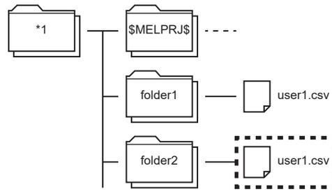
The file is not moved because a file with the same name exists in the destination. The SP.FCOPY instruction is finished normally. When there is not a file with the same name in the destination, the file is moved.
