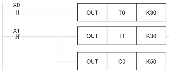
The set value of a timer or counter can be specified directly by a decimal number (K).
