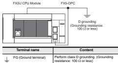
The connection destination for the FG terminal of FX5-OPC is a spring clamp terminal block. To connect to the terminal block, there are two ways; by usin single wires/strand wires or by using ferrules. Make sure to properly connect in accordance with the following specifications.
