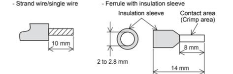
Check the shape of the wire insertion opening with the following chart, and use
