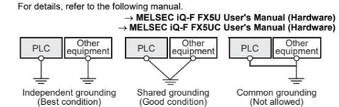
• Bring the grounding point close to the PLC as much as possible so that the ground cable can be shortened.
