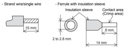
Check the shape of the wire insertion opening with the following chart, and use the smaller wire ferrule than the described size. Also, insert the wire with care so that the wire ferrule is in proper orientation. Failure to do so may cause the bite of the terminal and the damage of the terminal block.
