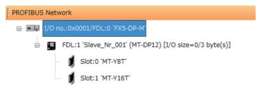
"Unregistered Program" that are auto generated when the PROFIBUS labels are updated are registered as "Scan". Create a program with the structures of these programs to enable I/O data to be assigned regardless of whether the data consists of a byte array or word array.
