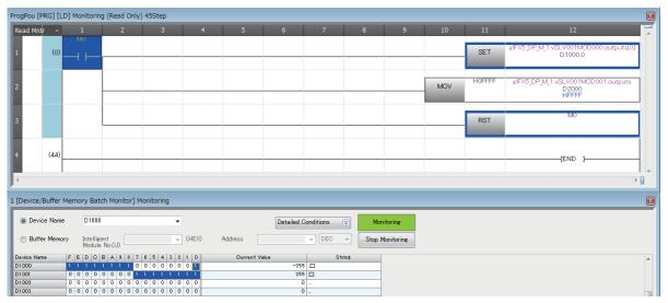
The data of Slot 1 MT-Y16T which have been divided in bit arrays are combined and stored as word arrays by iQFPBPOU\_1.
