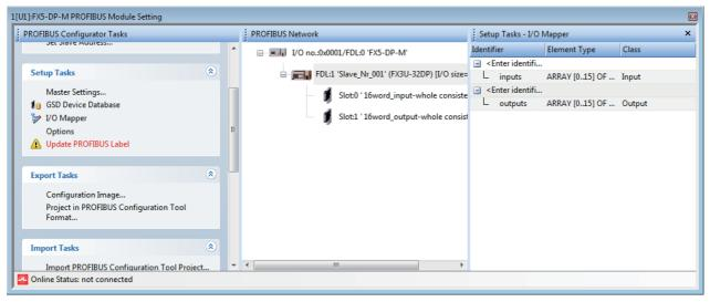
**3.** Edit the DUT elements. The DUT names and data types edited are applied in the DUT of global labels created when updating the PROFIBUS labels.
