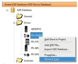
**2.** A confirmation window is displayed. Click the [Yes] button. The selected module is deleted from the GSD device database.
