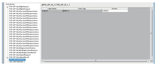
stSLV001\_MOD001\_1 is not assigned to the device but for two bytes of slot 1 MT-Y16T.
