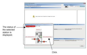
**4.** Cable test and remote operation can be performed by clicking the "Operation Test" or "Selected Station Operation" on the bottom right of the window. ( Page 119 Cable Test, Page 119 Remote Operation)
