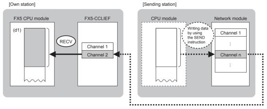
• The data received from the sending station is stored in the own station channel specified by the sending station and the corresponding bit in the GP.RECV instruction execution request area corresponding to each channel is set to on. When the corresponding bit in the GP.RECV instruction execution request area is set to on, the received data is read from the receive data storage channel. The following table lists the GP.RECV instruction execution request areas.
