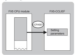
• The execution of the G(P).CCPASET instruction and whether it has been completed normally or completed with an error can be checked with the completion device (d) or completion status indication device (d)+1.
