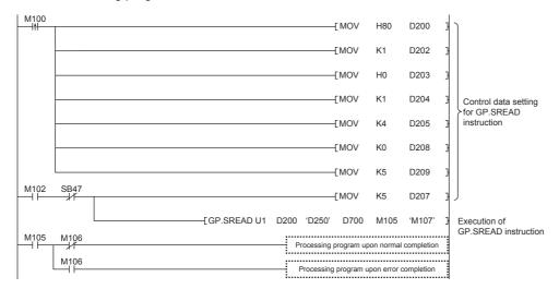
Write the following program to the CPU module of the target station of station No. 4.
