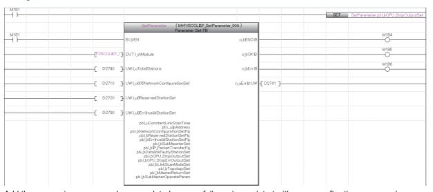
Add the processing program when completed successfully and completed with an error after the program above.
