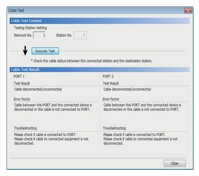
Click the [Cable Test] button in the "CC-Link IE Field Diagnostics" window.
