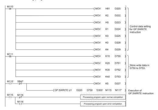
Write the following program to the CPU module of the target station of station No. 3.
