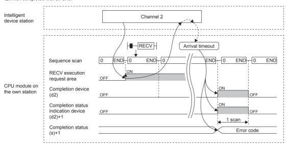
• Read processing is performed only once on the rising edge when the read command turns on.
