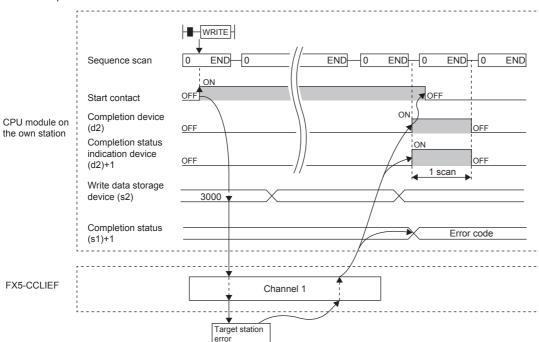
· Write processing is performed only once on the rising edge when the write command turns on.
