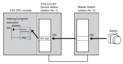
Set the interrupt setting parameters for the FX5-CCLIEF (station No. 1) in "Interrupt Settings" as shown below.
