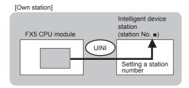
• The execution of the G(P).UINI instruction and whether it has been completed normally or completed with an error can be checked with the completion device (d) or completion status indication device (d)+1.
