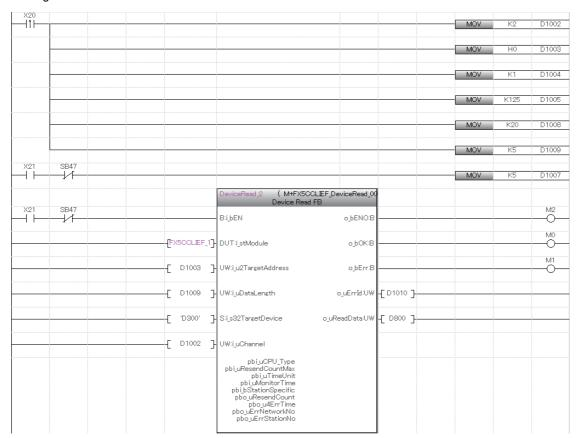
Add the processing program when read is completed and when completed successfully and completed with an error after the program above.
