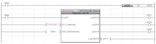
Add the processing program when completed successfully and completed with an error after the program above.
