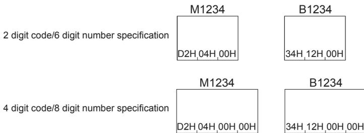
Internal relay M1234 becomes 0004D2H and is sent in the order of D2H, 04H, and 00H.
