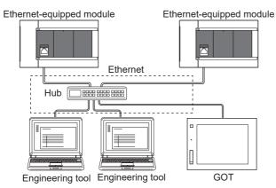
The flow up to start of Ethernet communication by the connection via a hub is as follows.
