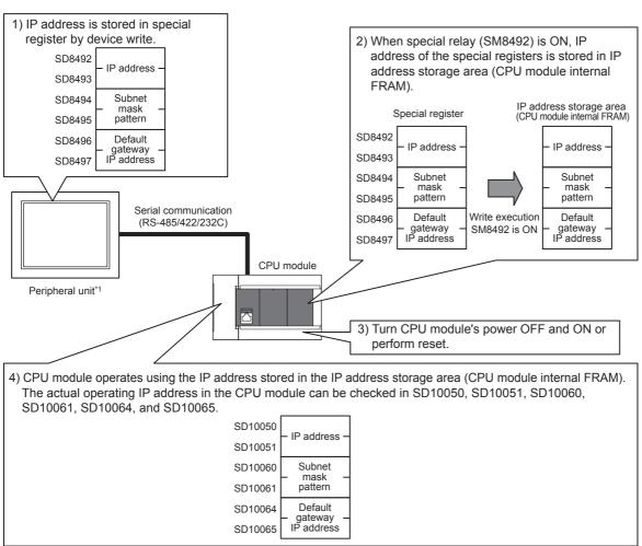
The IP address change function can be used not only by peripheral units but also by link function, MX Component and MX Sheet by manipulating values of the special devices. For details on link function, refer to the CMELSEC iQ-F FX5 User's Manual (Serial Communication). For details on MX Component and MX Sheet, refer to the respective product manual.
