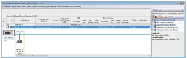
• Drag and drop the "Active Connection Module" from "Module List" to the left side on the window. Execute the settings as mentioned below.
