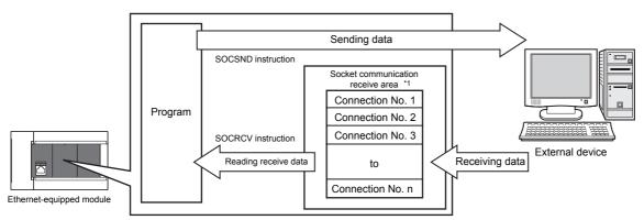
\*1 The area is used for storing data received from the connected open devices. CPU module: Connection No.1 to No.8 Ethernet module: Connection No.1 to No.32
