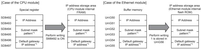
\*1 It is possible to specify no setting (0.0.0.0) for the subnet mask pattern and default gateway IP address. However, it is necessary to specify no setting (0.0.0.0) for both the subnet mask pattern and the default gateway IP address. If no setting (0.0.0.0) is specified for only one, an error will occur and the IP address will not be changed.
