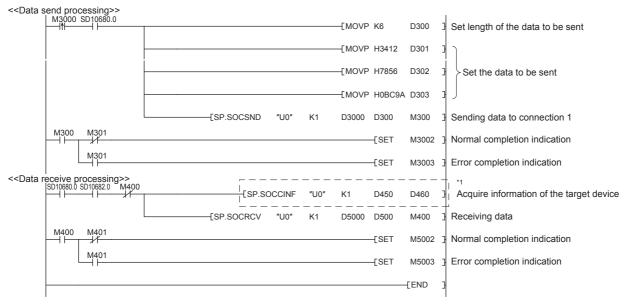
\*1 For acquiring information of the target device connected on UDP, run the program enclosed by the dotted line. (It can be omitted when the information acquisition is not needed.)
