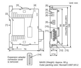
[1] DIN rail mounting groove (DIN rail: DIN46277, 35 mm wide)
