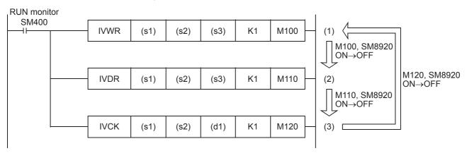
Inverter communication instructions standby for 11 ms after acquiring a serial port, and then starts communication. Even if
