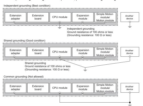
• Keep the distance between the grounding point and the programmable controller as close as possible to shorten the length of ground cable.
