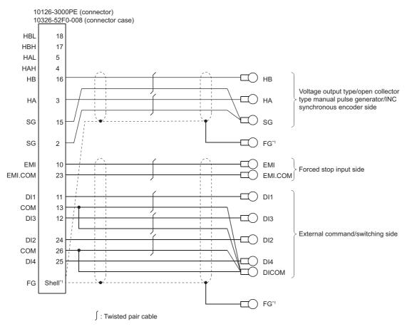
\*1 Make sure to perform shield treatment on the used equipment side. Also, connect it to the shell of connector side.
