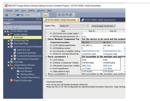
• The basic position information per rotation for the servo amplifier is 26 bit (67108864 pulse).
